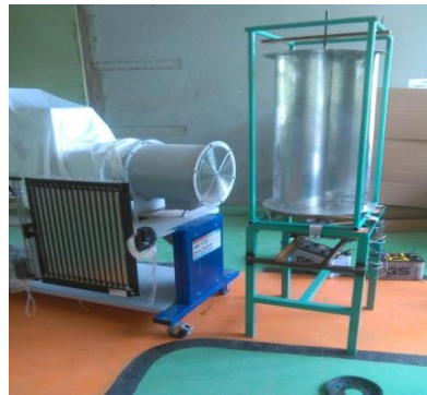
Figure 36: Testing the prototype using exhaust of the table top wind tunnel
