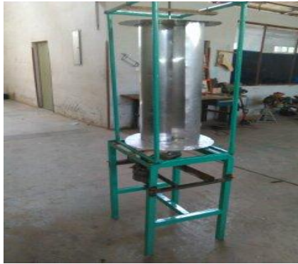
Figure 35: Assembled prototype Savonius vertical axis wind turbine rotor
