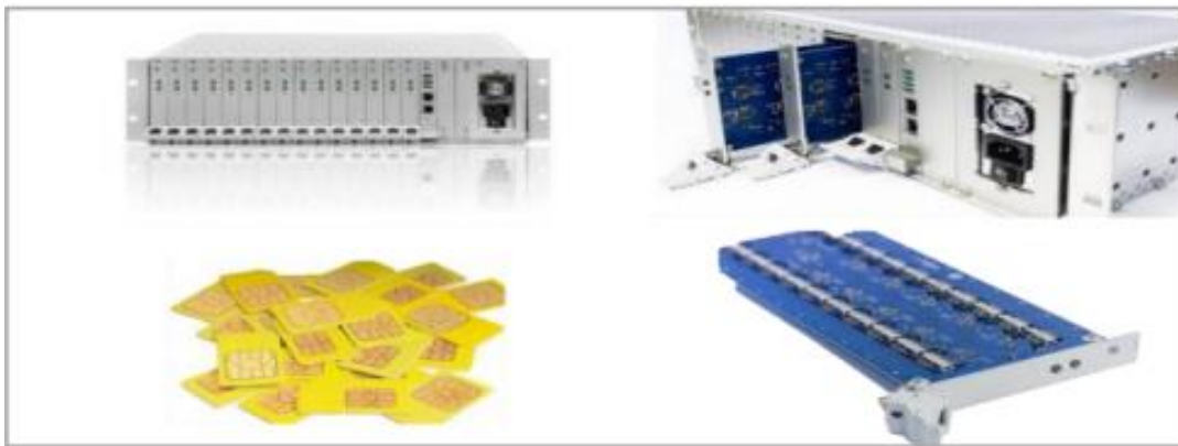
Figure 2.3 A SIMbox and its Components (Ighneiwa & Mohamed, 2017a)
