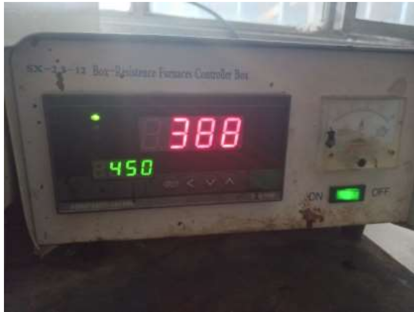
FIGURE 3 LABORATORY FURNACE USED FOR HEAT TREATMENT
