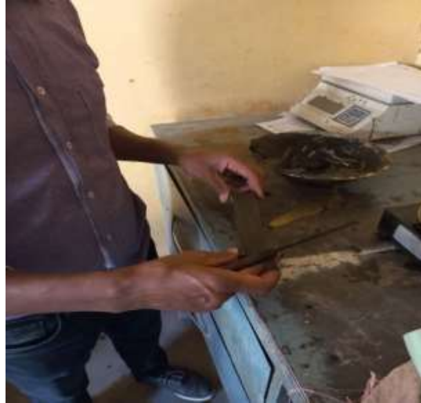
FIGURE 5 LINEAR SHRINKAGE TESTING
