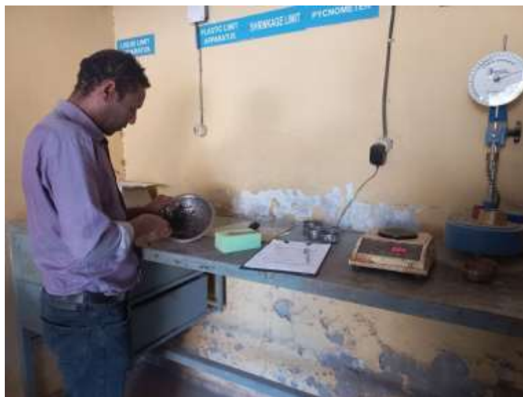
FIGURE 4 LABORATORY TESTING OF PLASTICITY OF SOIL
