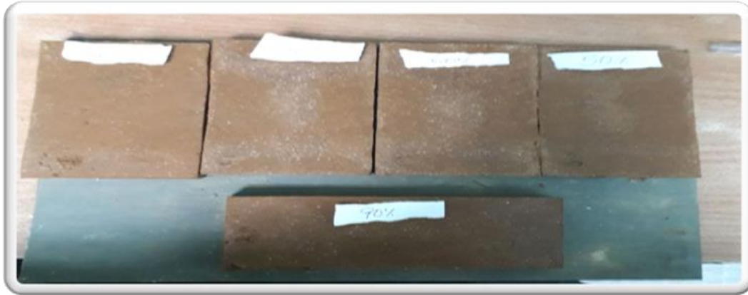
Figure 3.1: Pressed Sample of raw clay: Silica waste from AMWS (90:10, 80:20, 70:30, 60:40, 50:50)
