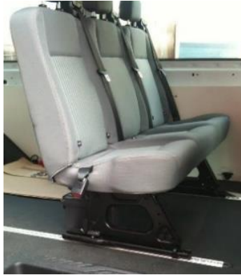
Figure 3-5 Example of previous seat direct contact with floor face
