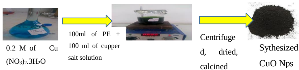
Figure 7: General procedure for the biosynthesis of copper oxide nanoparticles using Moringa stenopetala extract
