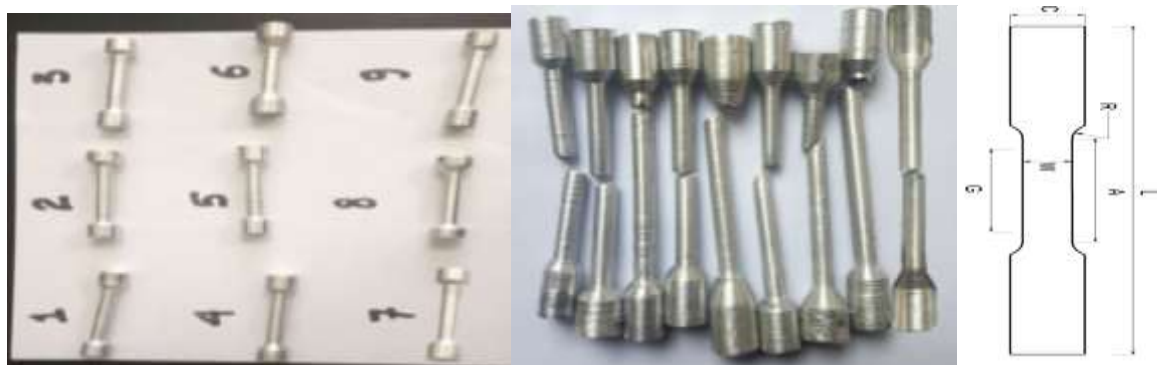
Figure 3.8: Sample before and after tensile testing and sample size
