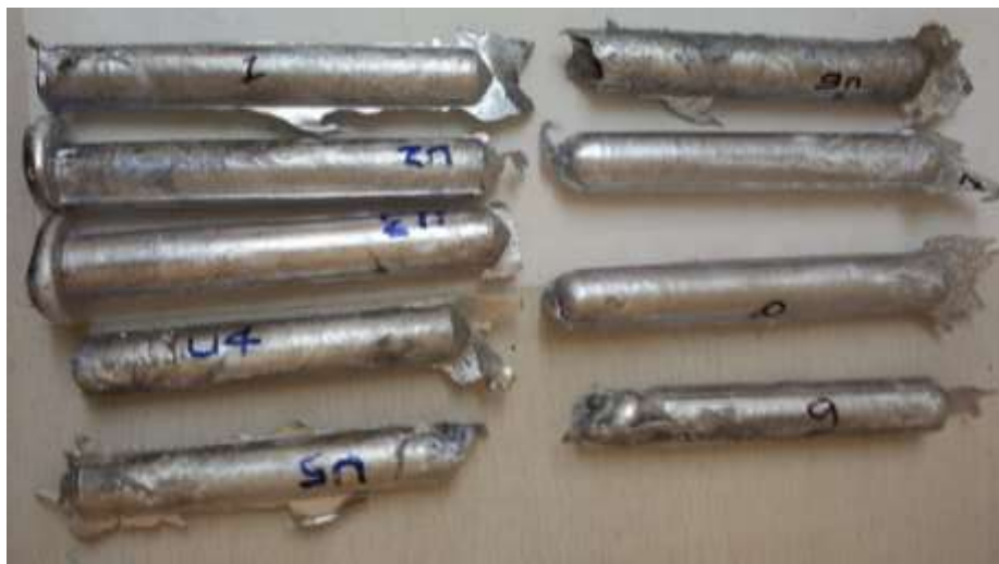
Figure 3.2: Cylindrical fabricated (casted) sample
