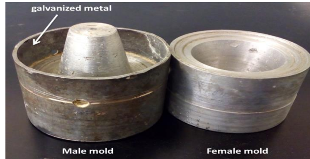
Figure 3. 9: Aluminum male (with galvanized metal outer cover) and female mold for CPWF forming
