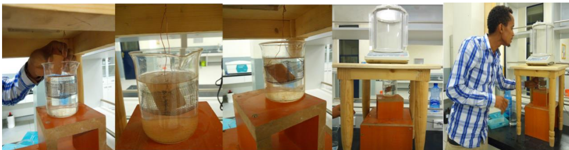
Figure 3. 7: Water absorption testing set up
