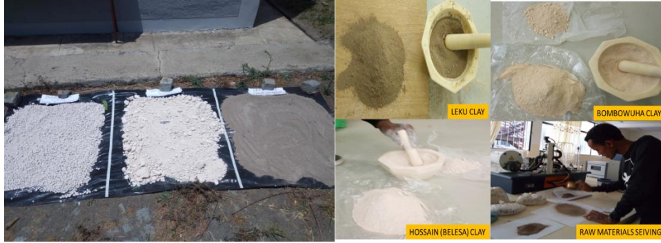
Figure 3. 1: Sun drying and beneficiation process of Bombowuha, Hosiana (Belessa) and Leku clay (left to the right respectively)
