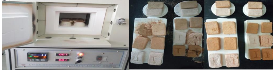
Figure 3. 5: Furnace firing of test bar samples and product of fired test bar samples at 800°C and 900°C from the left to right.
