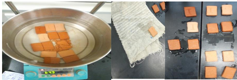
Figure 3. 6: boiling and drying of sample test bars (Archimedes liquid displacement method based on ASTM C373-88 (1988))
