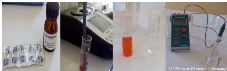
Figure 3. 15: Analyzing the fluoride concentration in raw ground water by using two kinds of fluorine reagent tablets under Photometer 7100 (wagtech, UK) and its PH value using 704 PH meter ( \Omega metrohm,Germany).
