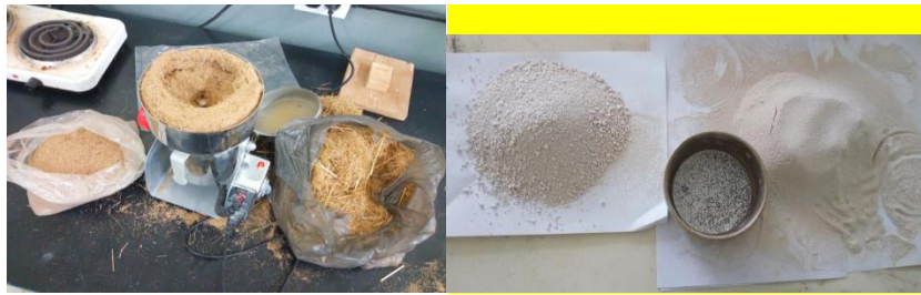
Figure 3. 8: Grinding and sieving of raw materials
