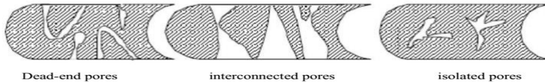
Figure 2. 4: Schematic diagram of the types of pores [22]
