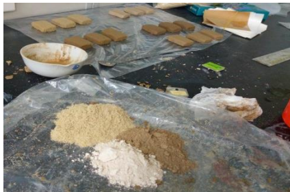
Figure 3. 2: Ready powders of Hossaina(the white) , leku clay(grey) and sawdust for dry mixng
