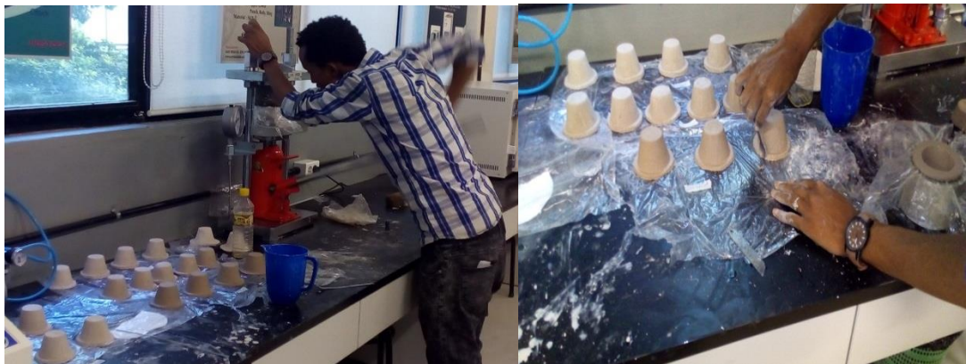
Figure 3. 10: Plastic forming of filter element by using semi dry clay to combustible plastic mix and surface finishing
