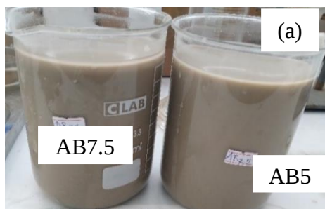
Activation of bentonite by \text{Na}_2\text{CO}_3
