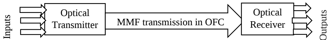
Figure 1.5. SDM using MMF in OFC systems (Puttnam, Rademacher, & Luís, 2021)
