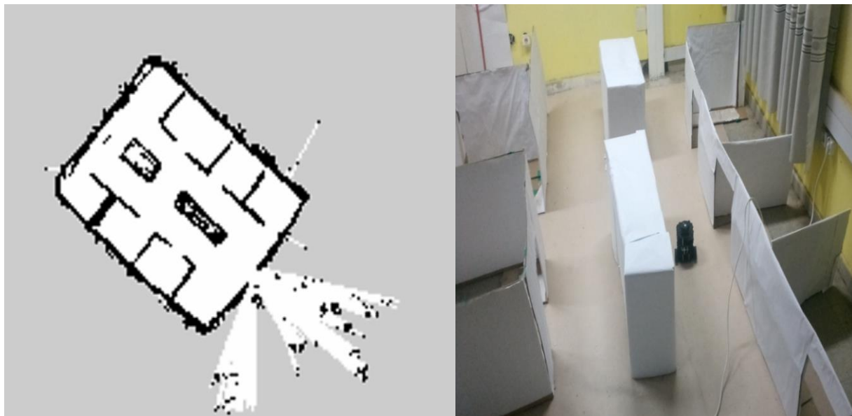
Figure 6. 12 Model built on real environment and the map built using Turtlebot3 LIDAR on rviZ
