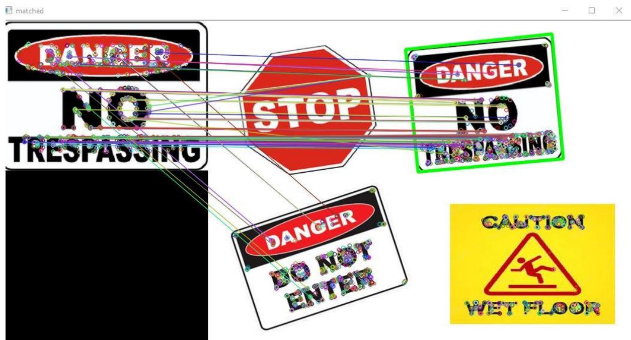
Figure 6. 9 Detecting the required image from different image by SURF+ORB
