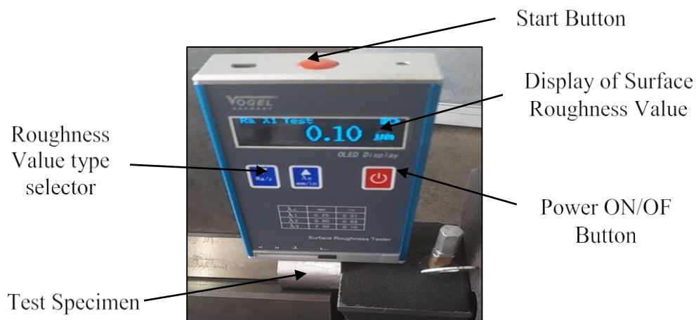
Figure 3-6: Surface-roughness testing equipment
