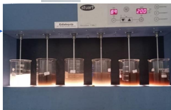
Adsorption process using CSH and \text{Fe}_3\text{O}_4 loaded CSH with different magnetite loading.
