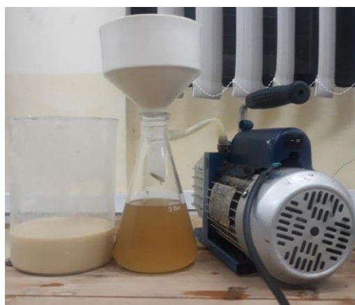
Separation of \text{Na}_2\text{SiO}_3 and Filter cake by Vacuum pump
