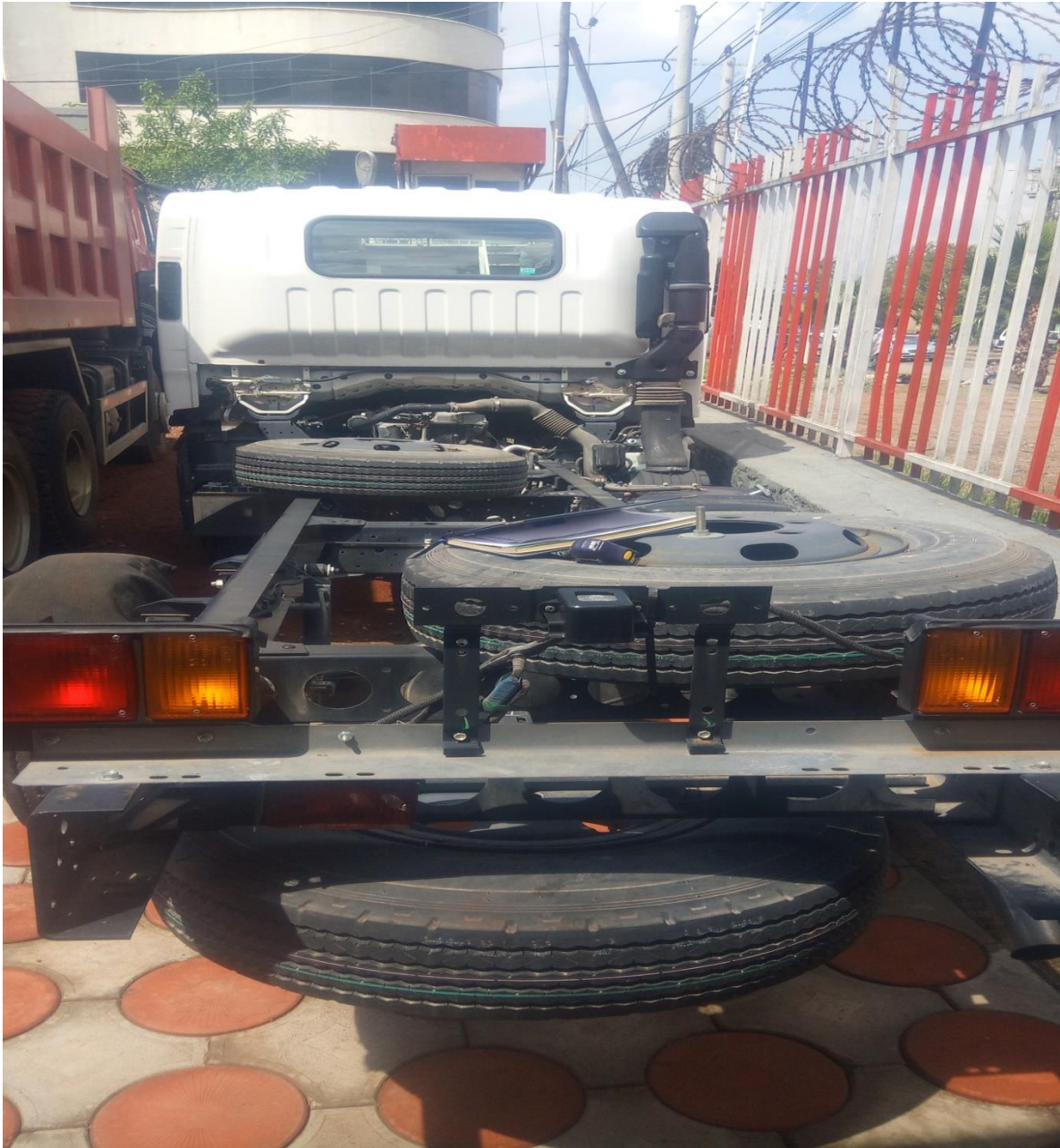
Figure A. 2: chassis frame of ISUZU- NPR vehicle.
