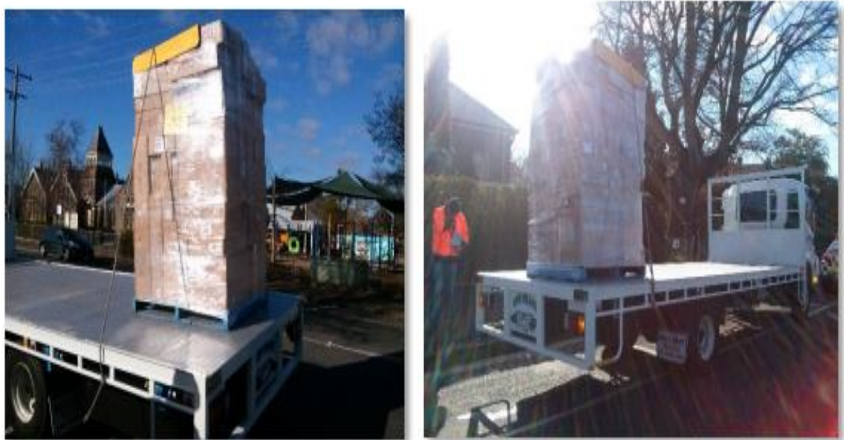
Figure 3. 18: Unbalanced load (poor loading) and load restraint practices.
