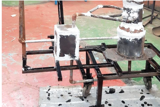
Figure 5.3. Constructed gasifier support frame
