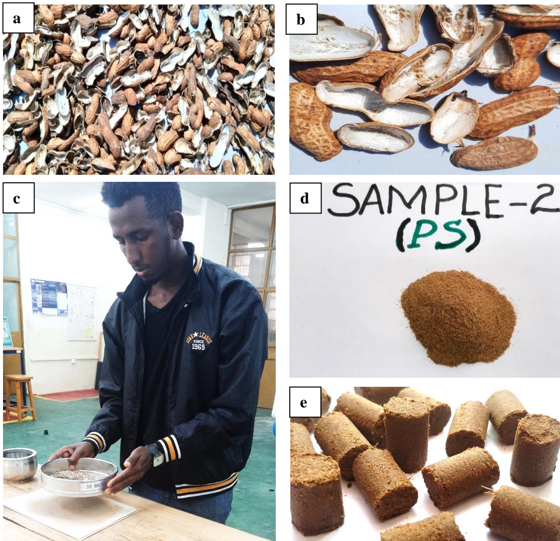
Figure C-2. PS preparation (a) sun drying (b) dried and cleaned PS (c) sieving (d) milled PS (e) PS pallets
