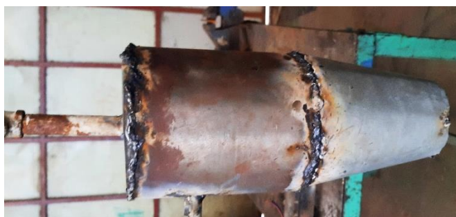
Figure 5.2. Fabricated cyclone separator
