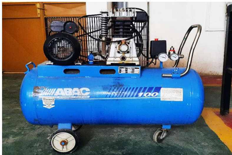
Figure G-2. Air compressor utilized for the gasifier
