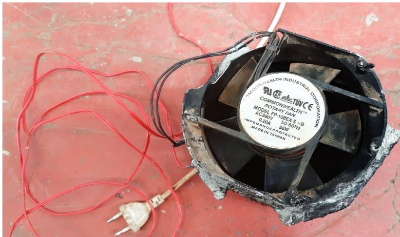
Figure G-1. Suction fan utilized for the gasifier
