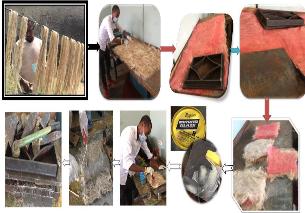
Figure 3.7: Banana fiber reinforced polymer composite fabrication procedures
