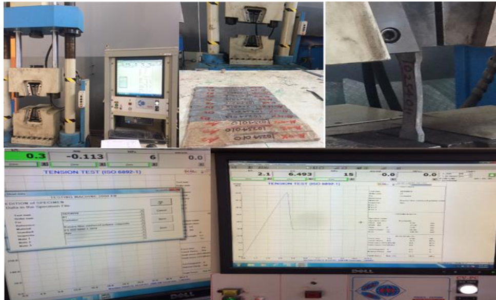
Figure 3.11: UTM-2000kN used to test tensile stress
