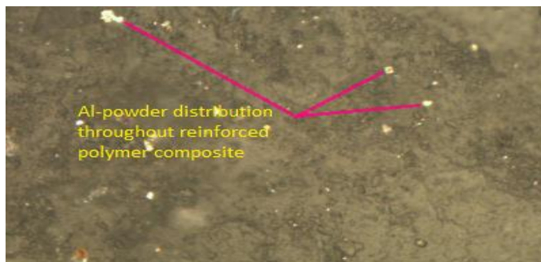
Figure 4.7: Microstructure of sample B
