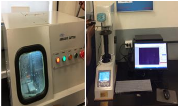
Figure 3.13: Abrasive cutting in action (RB-203), Micro-hardness measurement under Vickers Hardness Tester (HVS-50)
