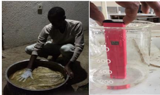
Figure 3.5: Banana fiber treatment in 5% NaOH solution and its PH measurement
