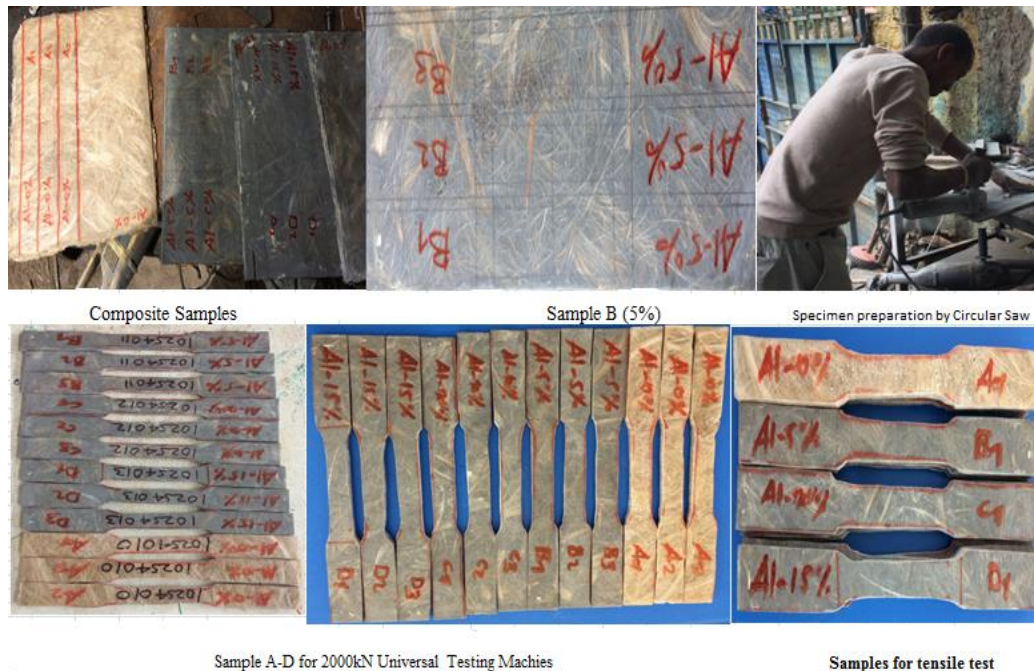
Figure 3.10: Specimen identification codes (User's code) for tensile test on UTM-2000kN
