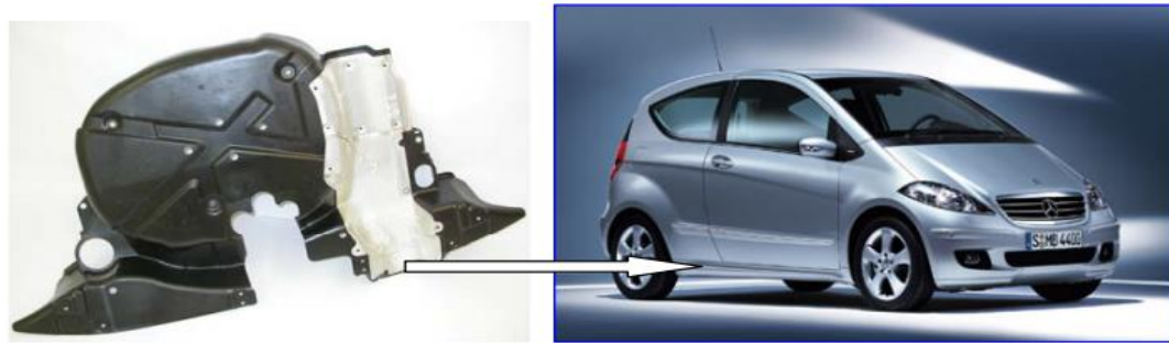
Figure 2.7: Under floor protection trim of Mercedes A Class made from Banana fiber reinforced composite
