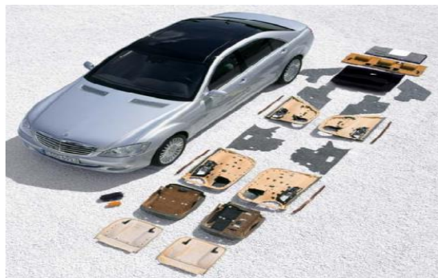
Figure 2.8: Newest Mercedes S Class Automotive components made from different bio fiber reinforced components
