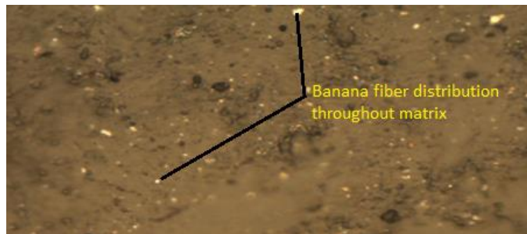
Figure 4.6: Microstructure of Sample A
