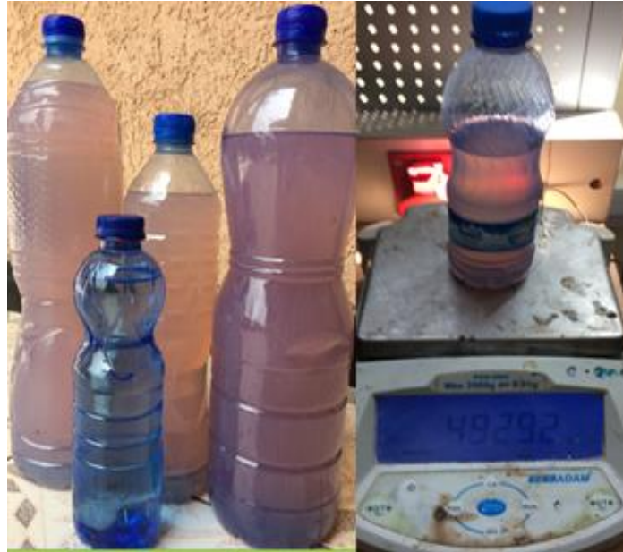
Figure 3.4: Resin and hardener measurement on digital balance by weight fraction
