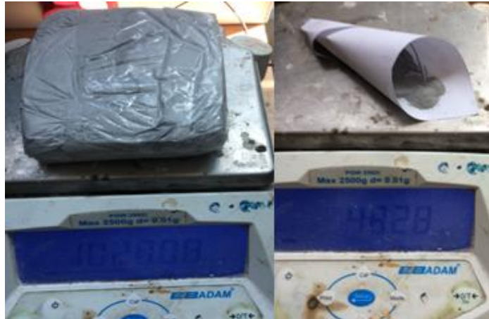
Figure 3.3: Al-powder filler measuring on digital balance based on weight ratio
