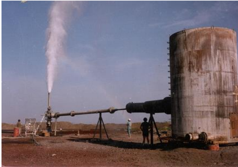
Figure 15: One of the shallow wells (TD-5) of the Tendaho Geothermal Field, total depth and maximum temperature of 516 m and 253°C, respectively (Kebede et al.,2010).
