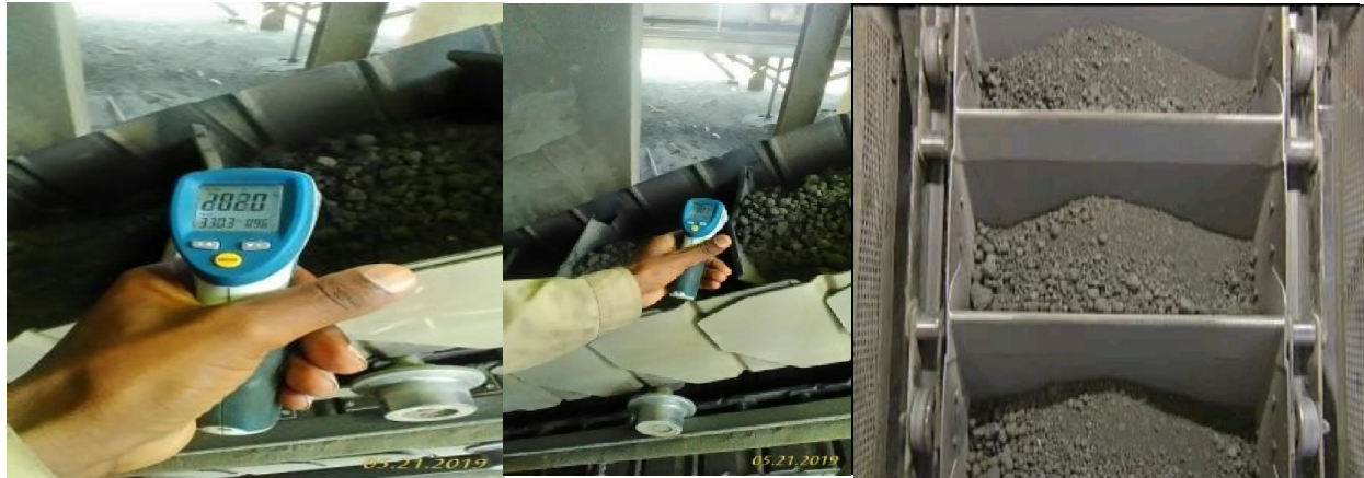
Figure 5.3 Measured temperature of outlet clinker by Dual Leaser Infrared Thermometer
