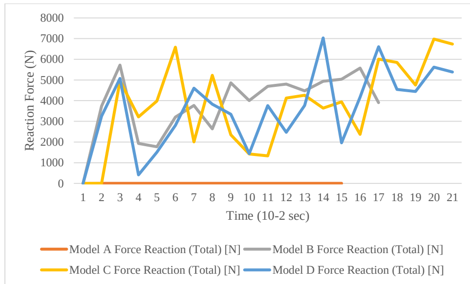
Figure 4.2: Comparison of total reaction forces of all models (Model A, B, C, and D)
