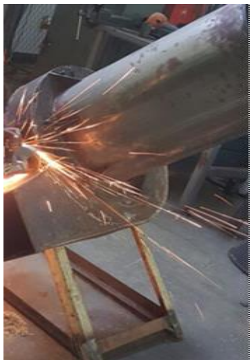
Figure 6. Modification and fixing of the outlet of the machine
