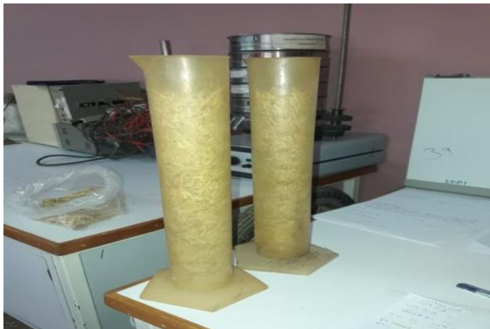
Figure 3.29. Determination of bulk density of grinded straw
