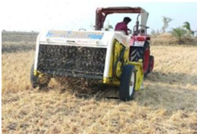
Figure 2.5. Tractor operated straw leftover chopper and spreader machine
