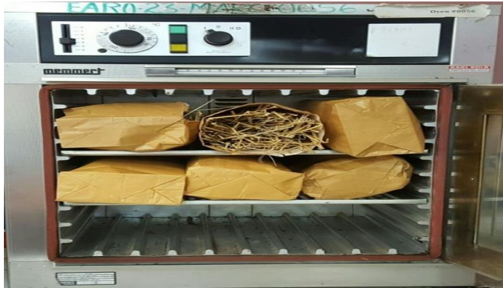
Figure 3.30. Measuring moisture content of the sample with oven method.
