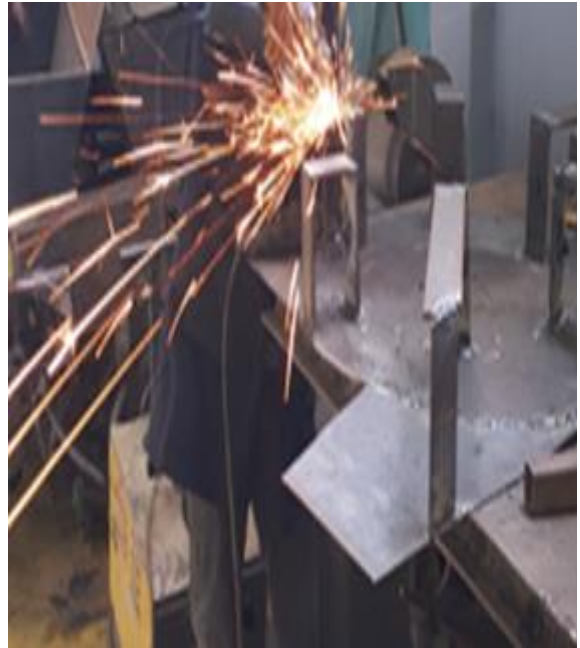
Figure 2. Part welding and surface grinding
