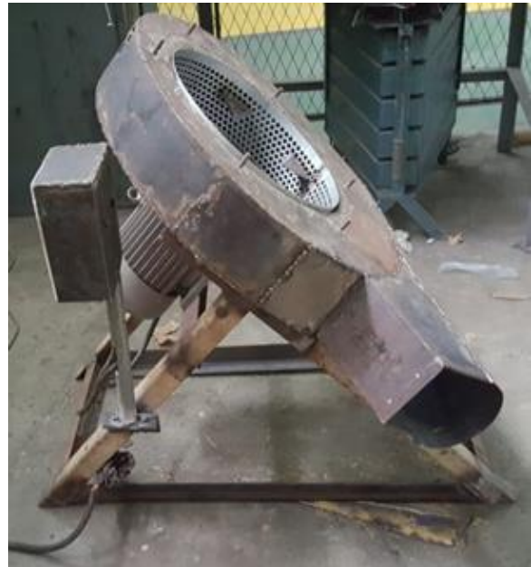
Figure 4. Partial assembling of the machine on the frame
