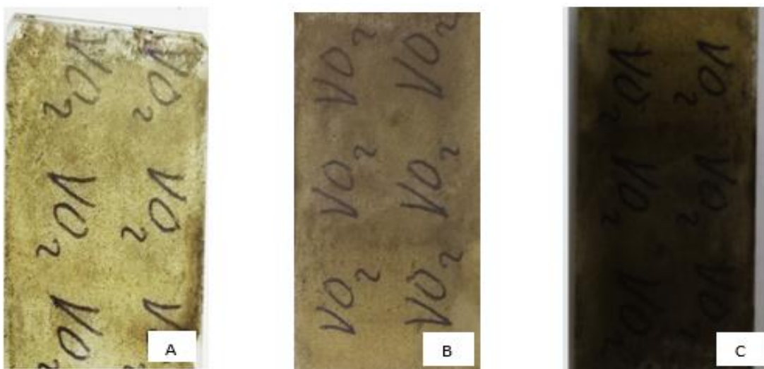
Figure 3.8: Showing thin films after annealing at 570 °C for 2 h a)15 minute b)30 minute c) 80 minute deposition times.
