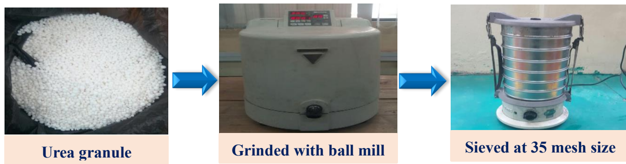
Figure 3.4. Urea powder preparation
