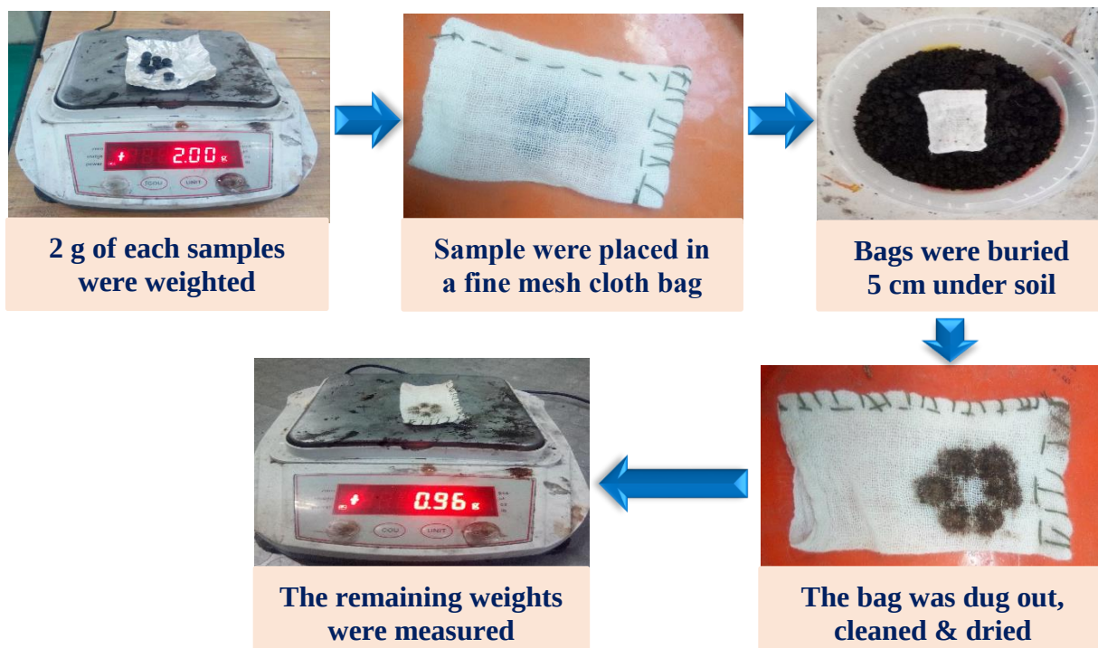
Figure 3.8. Soil degradation test process of U-e-LAO-g-GAs and commercial urea
