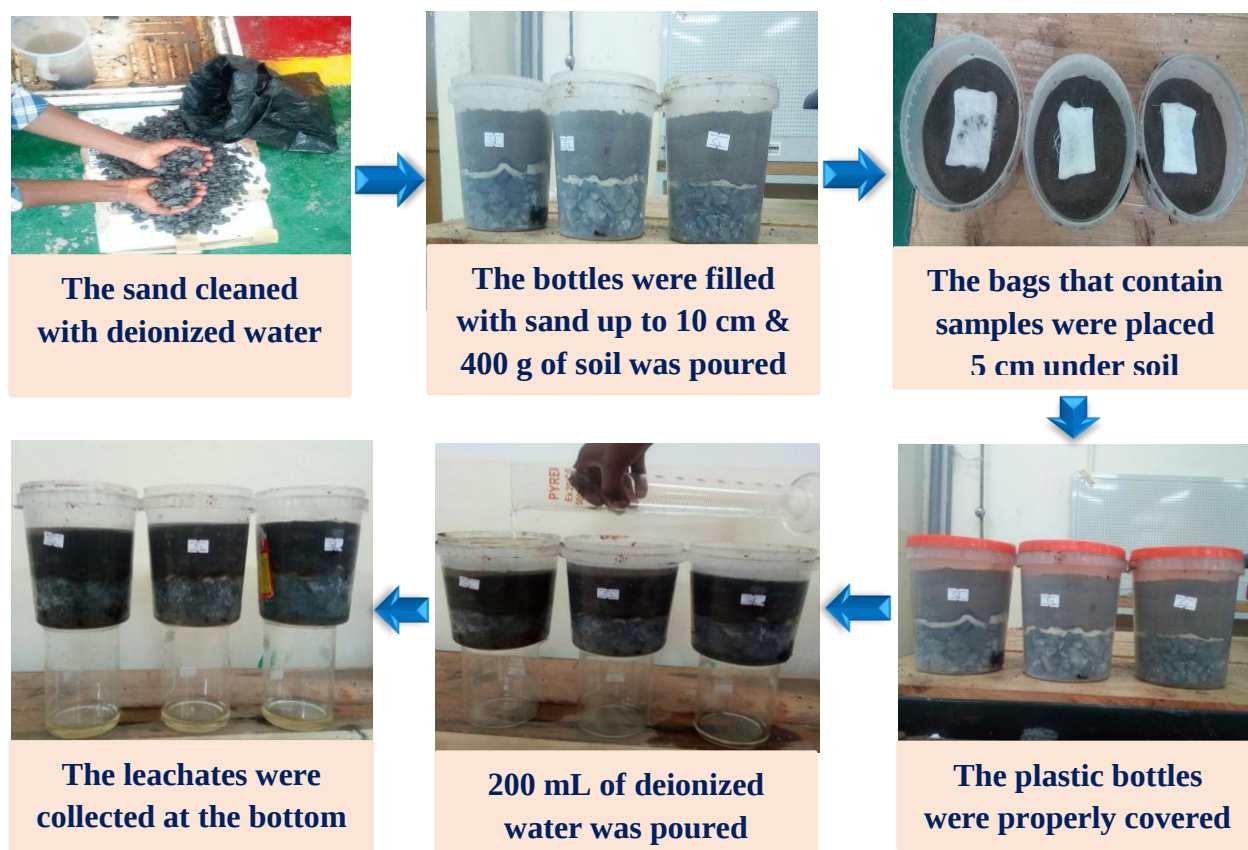
Figure 3.7. Experimental procedure to determine urea release rate of samples in soil
