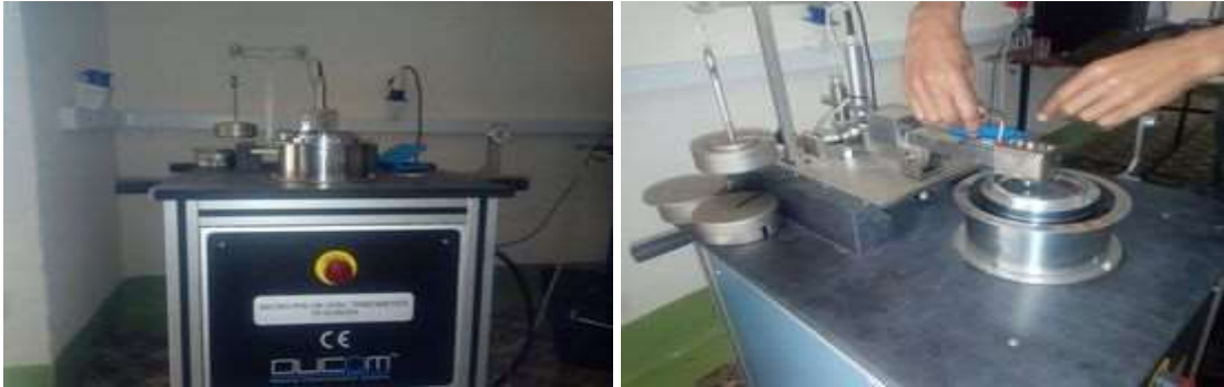
Figure 3.13. Wear rate test set up
