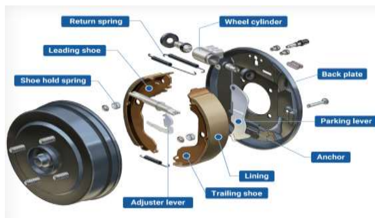
Figure 2.3. Main components of drum brake ( https://www.fahadhvhassan.com/drum-brake-function-components-working-principle-and-types )
