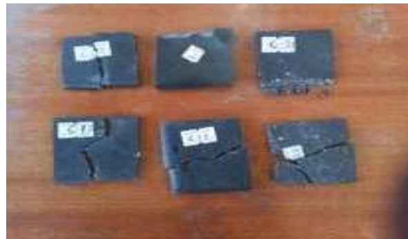
Figure 4.5. Composite samples after compression test
