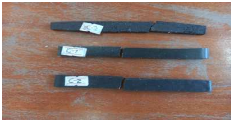
Figure 4.10. Sample after flexural test
