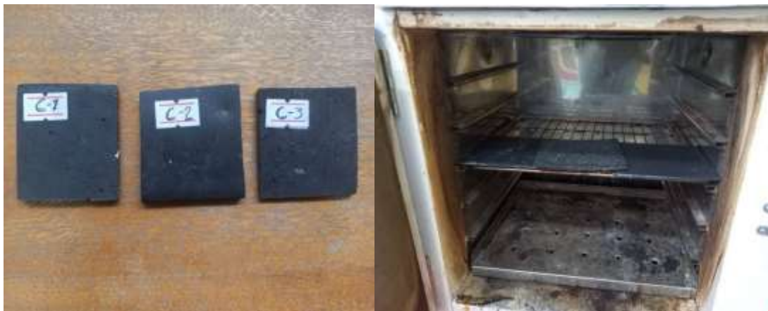
Figure 3.6. (a) Composite samples and (b) curing process
