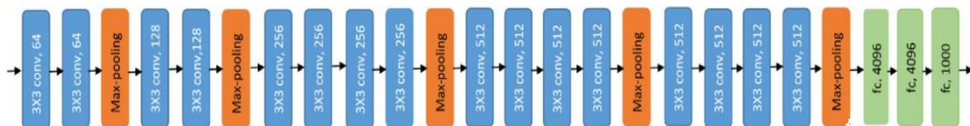
Figure 2 Schematic Architecture of VGG-19 Pretrained model
