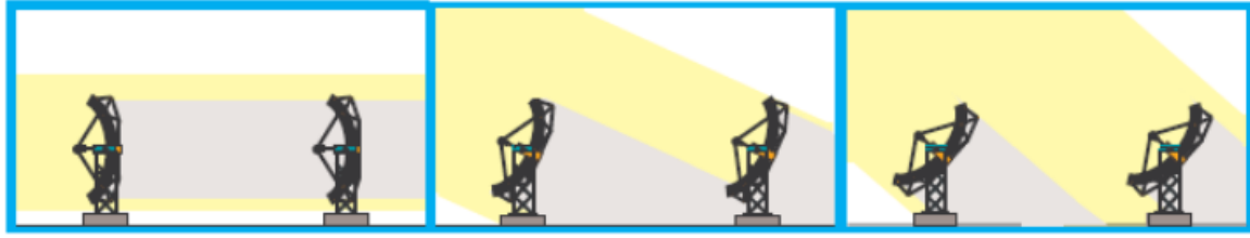
Figure 4- 5: Collector tracking through morning, showing digression of collector shading as the day progresses (Assefa,2011).
