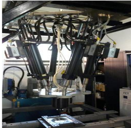
Figure 2. 3 Prototype machine for SPIF from University of Aveiro Yau, (2001).
