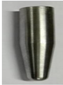
Figure 3. 4 Hemispherical forming tool with 15 diameters tip
