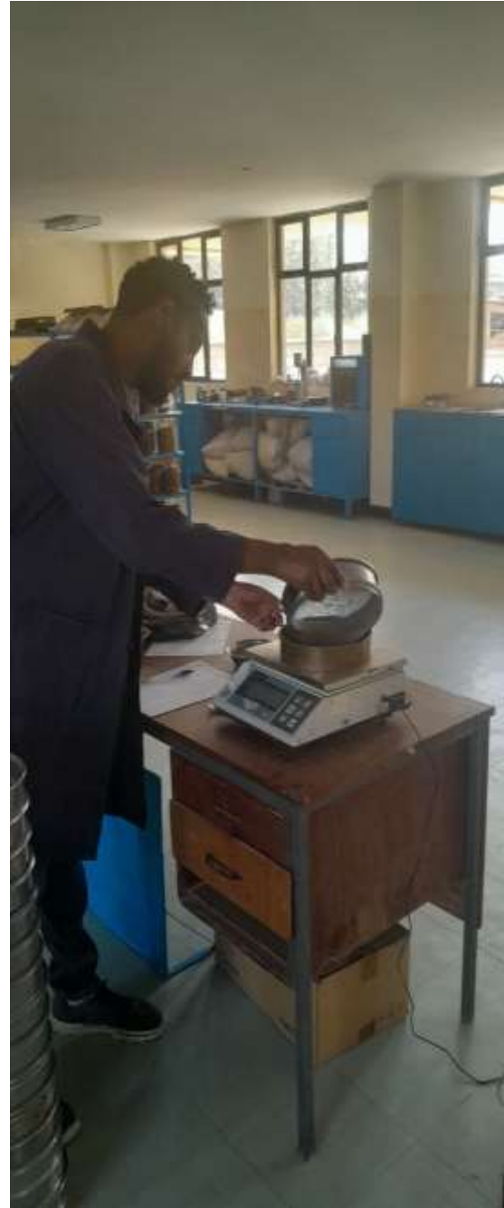
Figure 3.13: During weighting and Sieving of a sample(Reference Gondwana Engineering)
