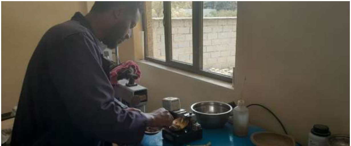
Figure 3.14: During Liquid Limit determination. (Reference Gondwana Engineering)
