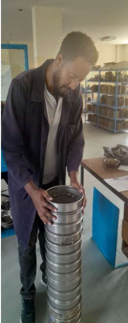
Figure 3.13: During weighting and Sieving of a sample(Reference Gondwana Engineering)
