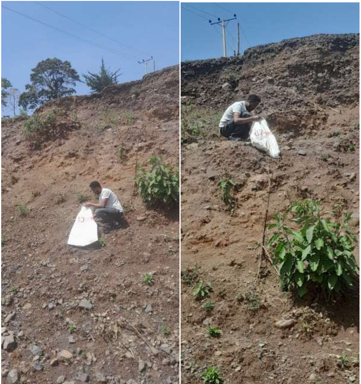
Figure 3.12: Sampling of Disturbed Soil at different depths of Site 7 at station 104+140
