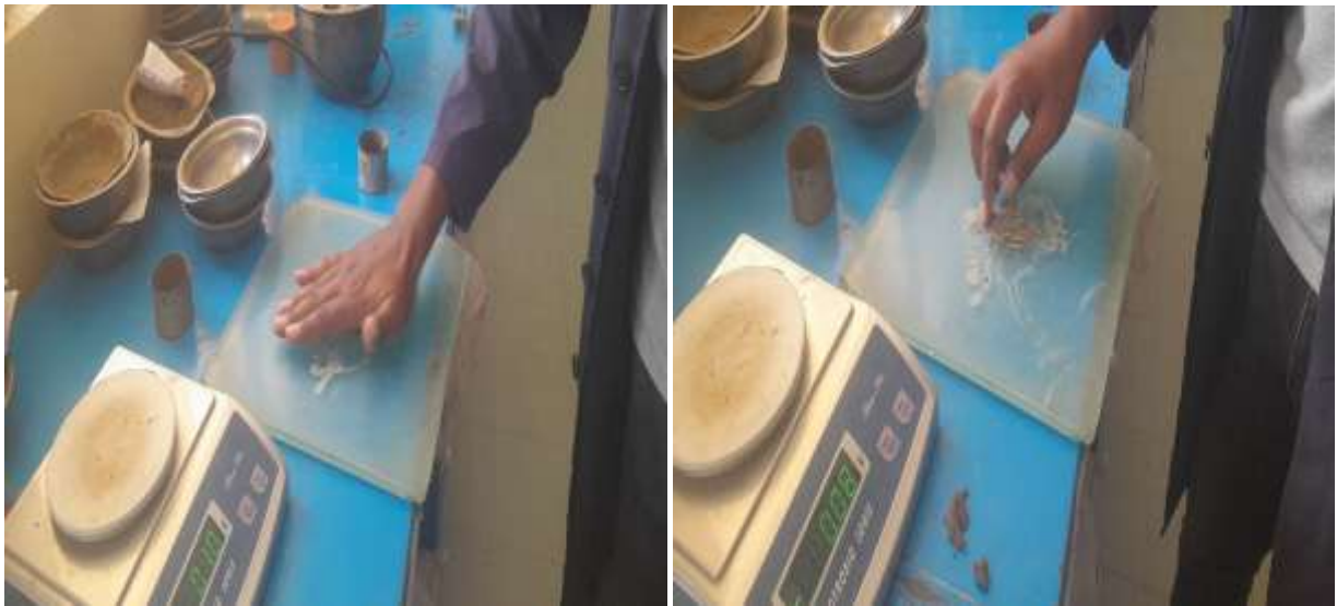
Figure 3.15: During Plastic Limit determination(Reference Gondwana Engineering).
