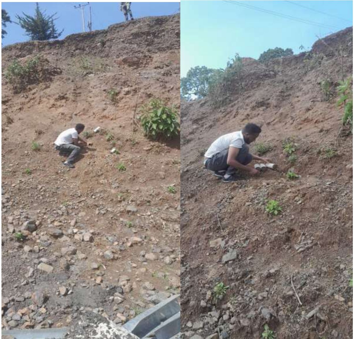
Figure 3.11: Sample of Undisturbed Soil at different depths of Site 7 at station 104+140
