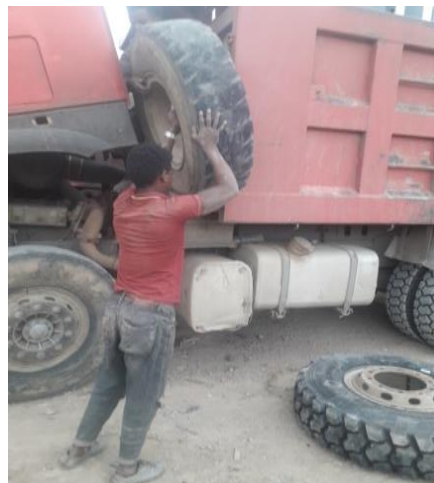
Figure 1.2: Lowering spare tyre
