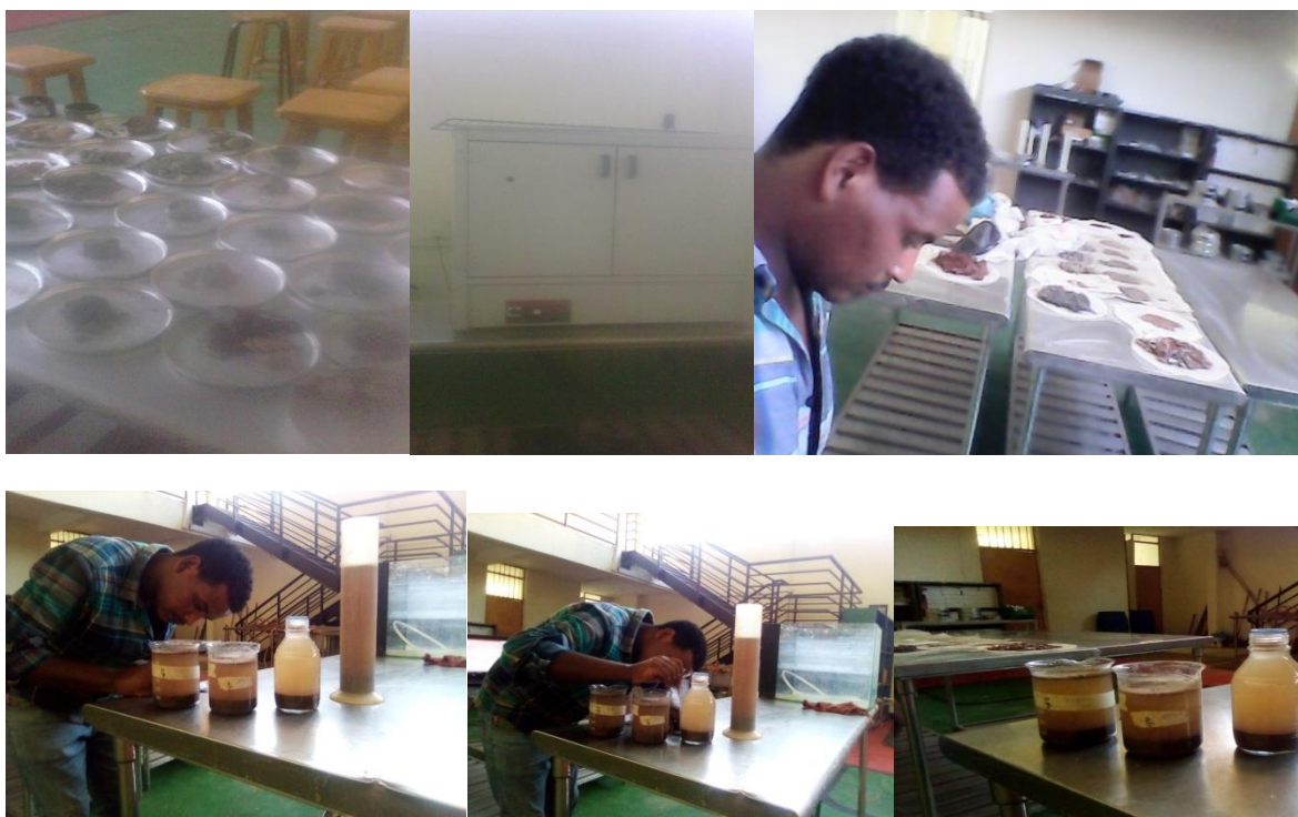
Figure 3.2: Initial soil moisture and textural class laboratory determination by photo in Civil Department Adama Science and Technology University Soil laboratory.
