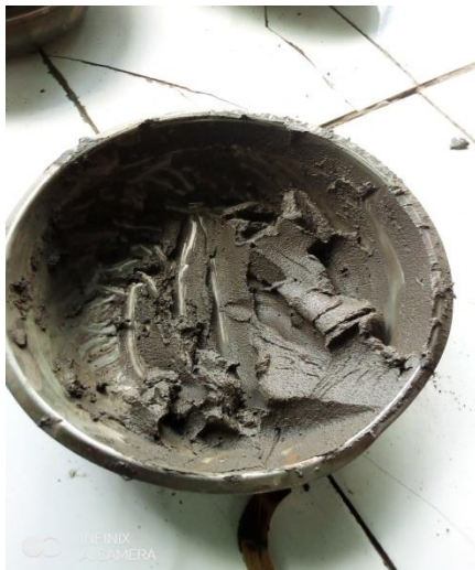
Figure I.6 Linear shrinkage process a) mixing of sample, b) filling wet sample with mould c) sample prepared for drying
