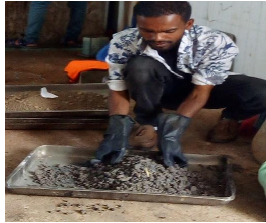
Figure I.2 Modified proctor compaction a) sample prepared, b) compaction operation
