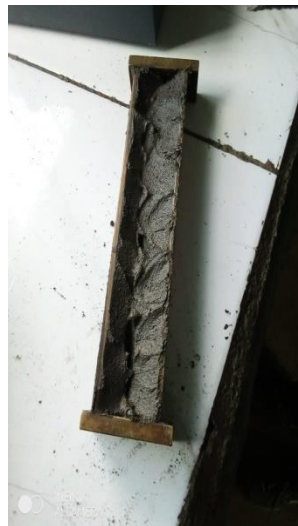
Figure I.6 Linear shrinkage process a) mixing of sample, b) filling wet sample with mould c) sample prepared for drying
