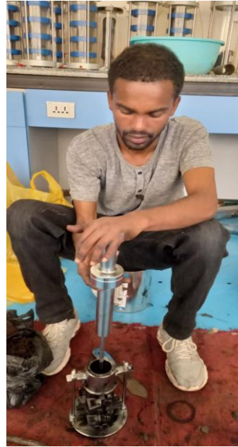
Figure I.7 Unconfined compressive strength a) remolded specimen b) tamping the soil c) UCS loading machine
