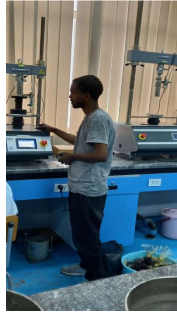
Figure I.7 Unconfined compressive strength a) remolded specimen b) tamping the soil c) UCS loading machine
