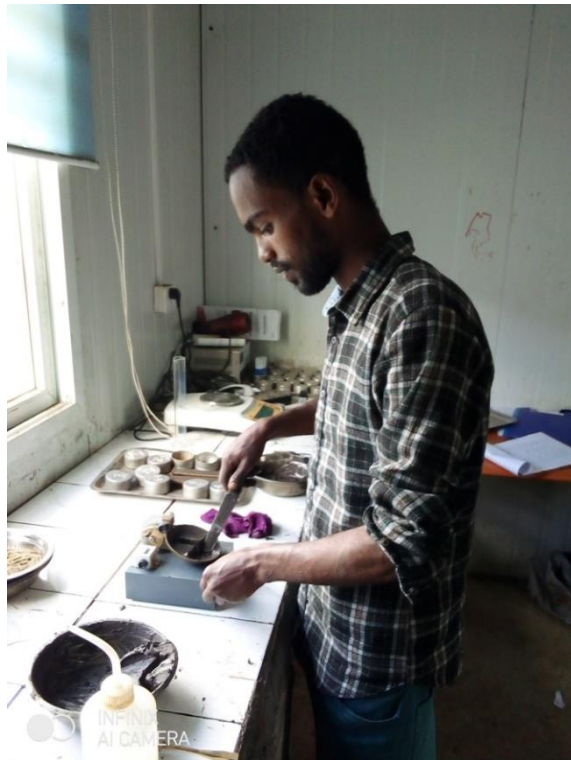
Figure I.1 Determination of Atterberg limits
