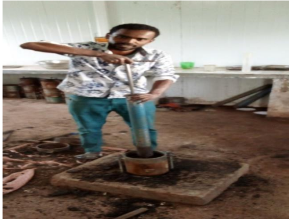
Figure I.2 Modified proctor compaction a) sample prepared, b) compaction operation
