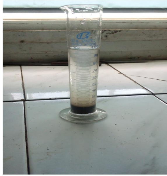
Figure I.5 Free swell test process
