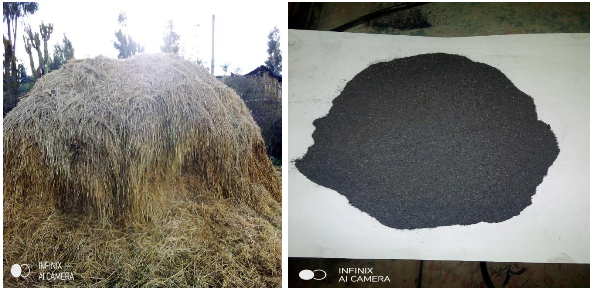
Figure 3.5 WHA before burning and after burning.
