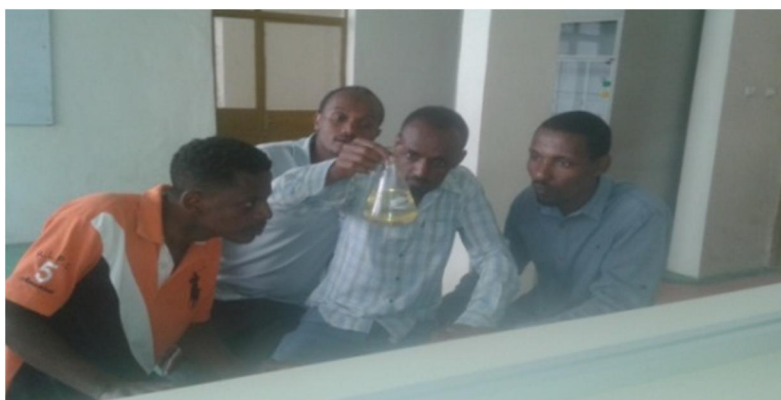
Figure 5.1 Checking phase separation of gasoline, ethanol and methanol blend
