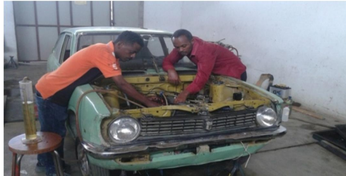
Figure 4.4 Ignition timing adjustment
