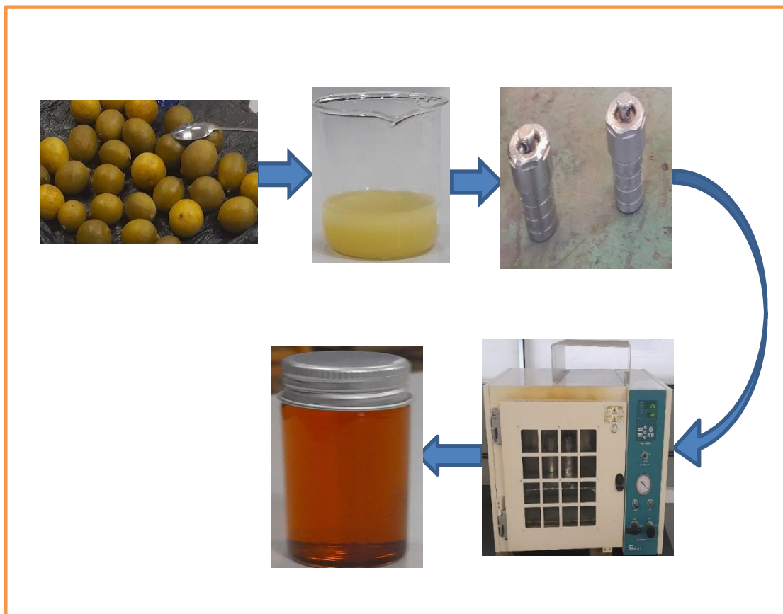
Figure 3. 1: Show a schematic of the synthesis of carbon quantum dots (CQDs) from lemon juice using hydrothermal techniques.
