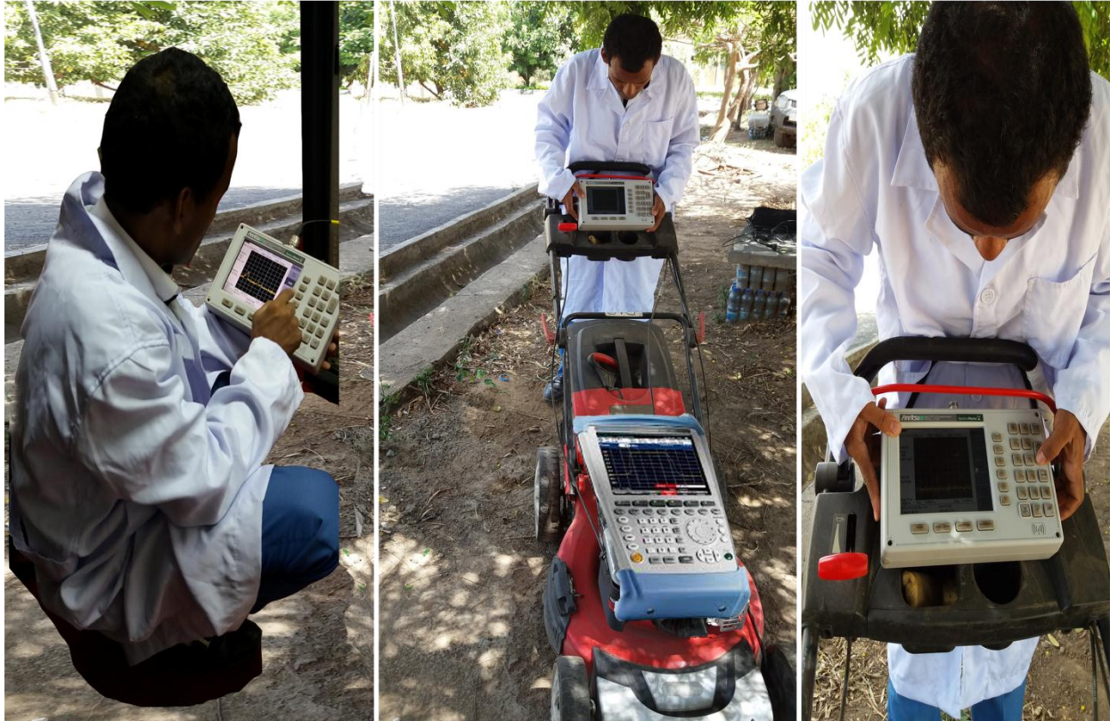
Figure. 5.7. Taking Measurement with Ground Penetrating Radar at site
