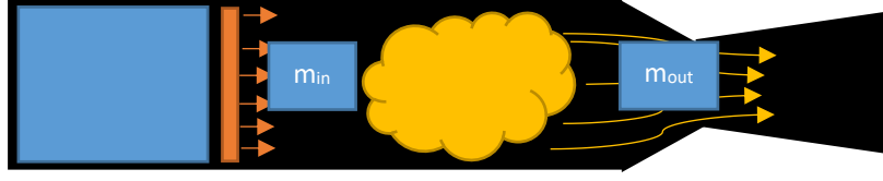
Figure 23: Mass balance in combustion chamber
