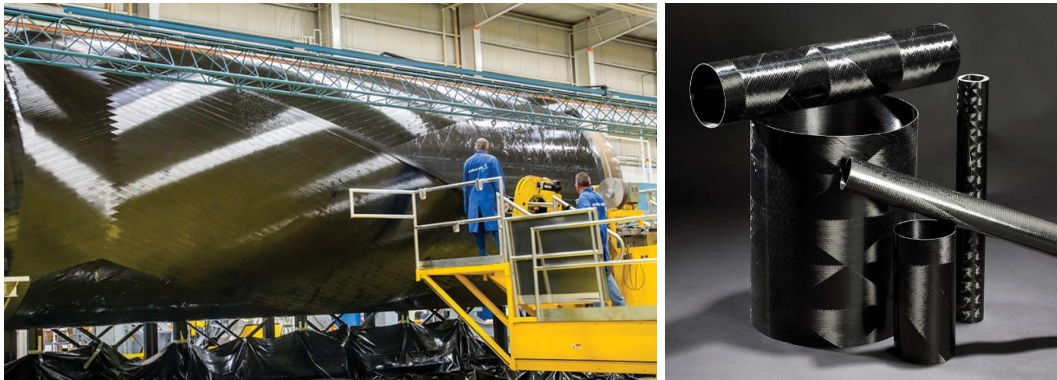
Figure 6: Filament wound composites for rocket motor cases (Mateduc Composites, n.d.)
