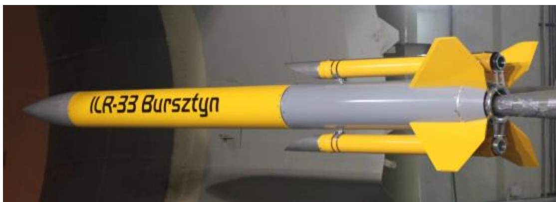
Figure 8: Full-scale mockup of the ILR-33 “Amber” sounding rocket.(Nowakowski et al., 2017)
