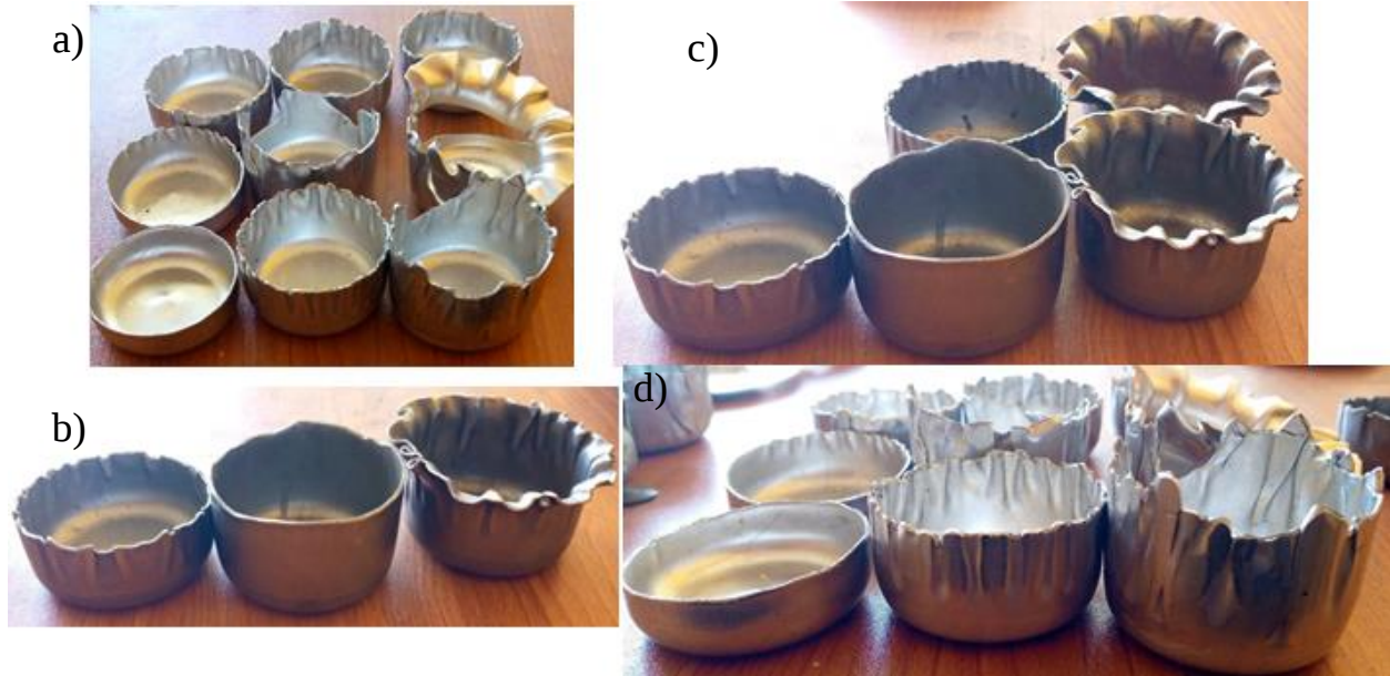
Figure 4. 5: Deep drawn cups with different blank holding force; fig. a & d shows deep drawn cup for AA6061 and fig. c & b shows deep drawn cup for Low-carbon steel sheet
