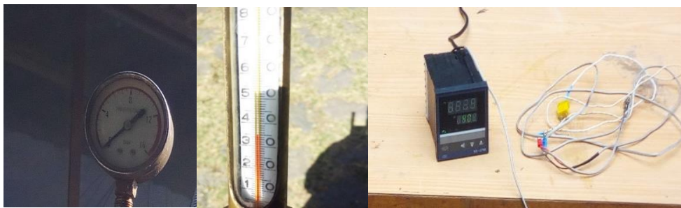
Figure 4.16: Measuring instrument Pressure gauge, thermometer, Thermocouple
