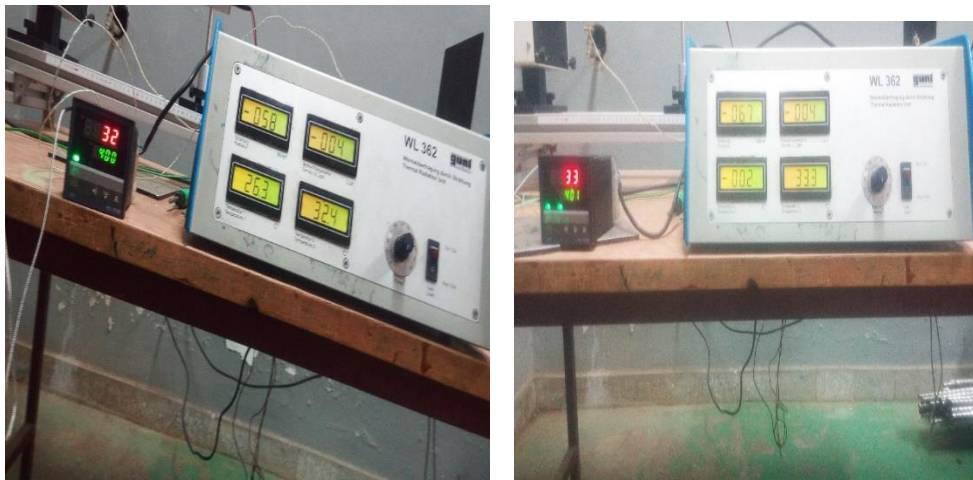
Figure C. 1. Thermocouple Calibration with The Standard
