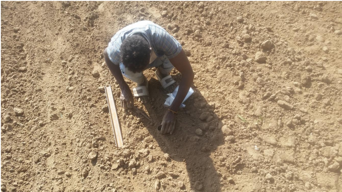
Figure.G.4. Picture showing taking of soil sample to measure soil moisture content and bulk density
