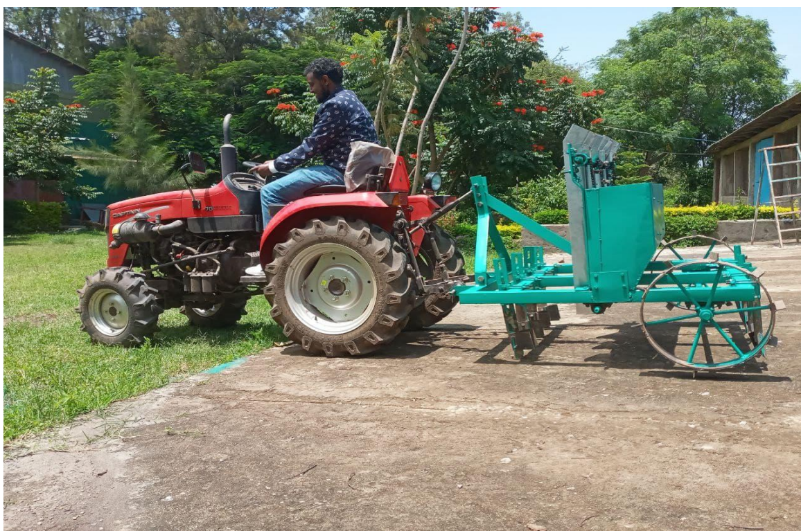
Figure 4.1. Calibration of garlic planter
