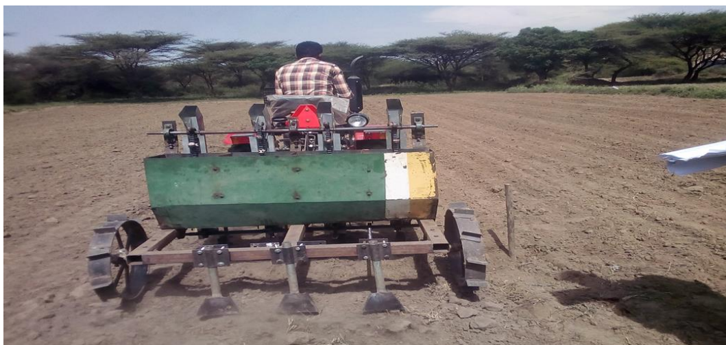
Figure 4.4. Garlic planter under operation
