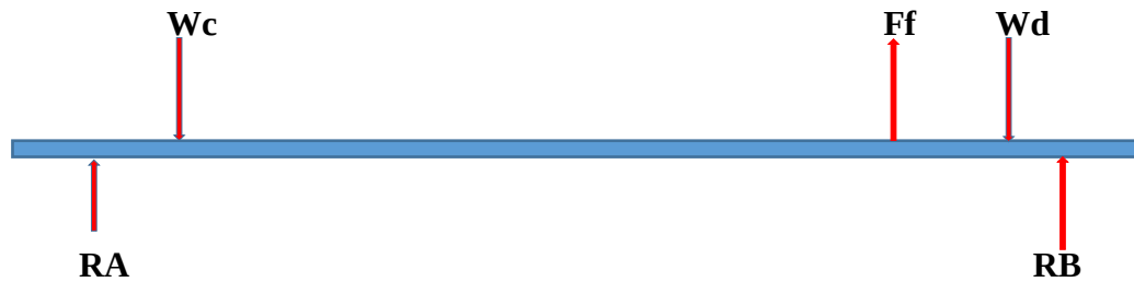
Figure 3.11. Vertical force distribution on the shaft
