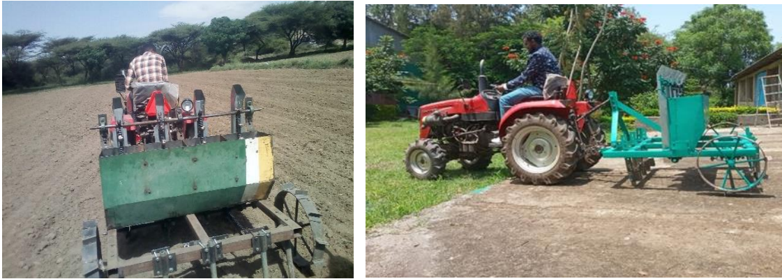
Figure G.5. Picture shows data taking during Performance evaluation of tractor drawn garlic planter
