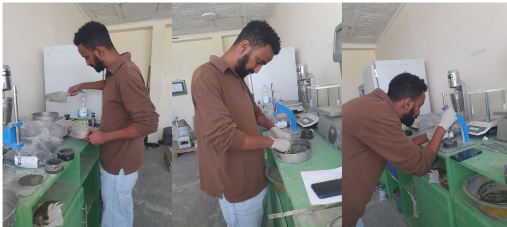
Figure 3-0-15 Consistency of cement test
