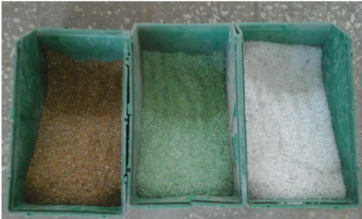
Figure 4.8 fine aggregate made from different color of waste glass/bottles/
