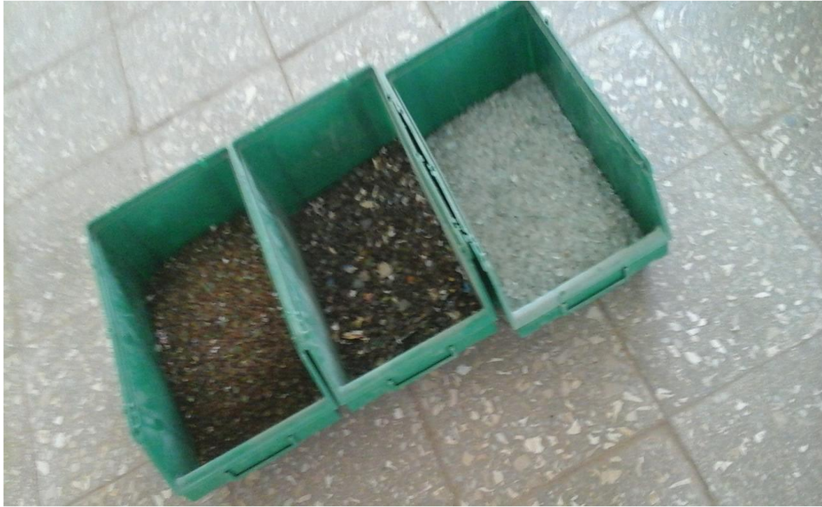
Figure 4.7 coarse aggregate made from different color of waste glass/bottles/
