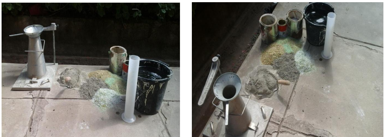
Figure 4.13 Raw materials and equipments used for slump test of the project
