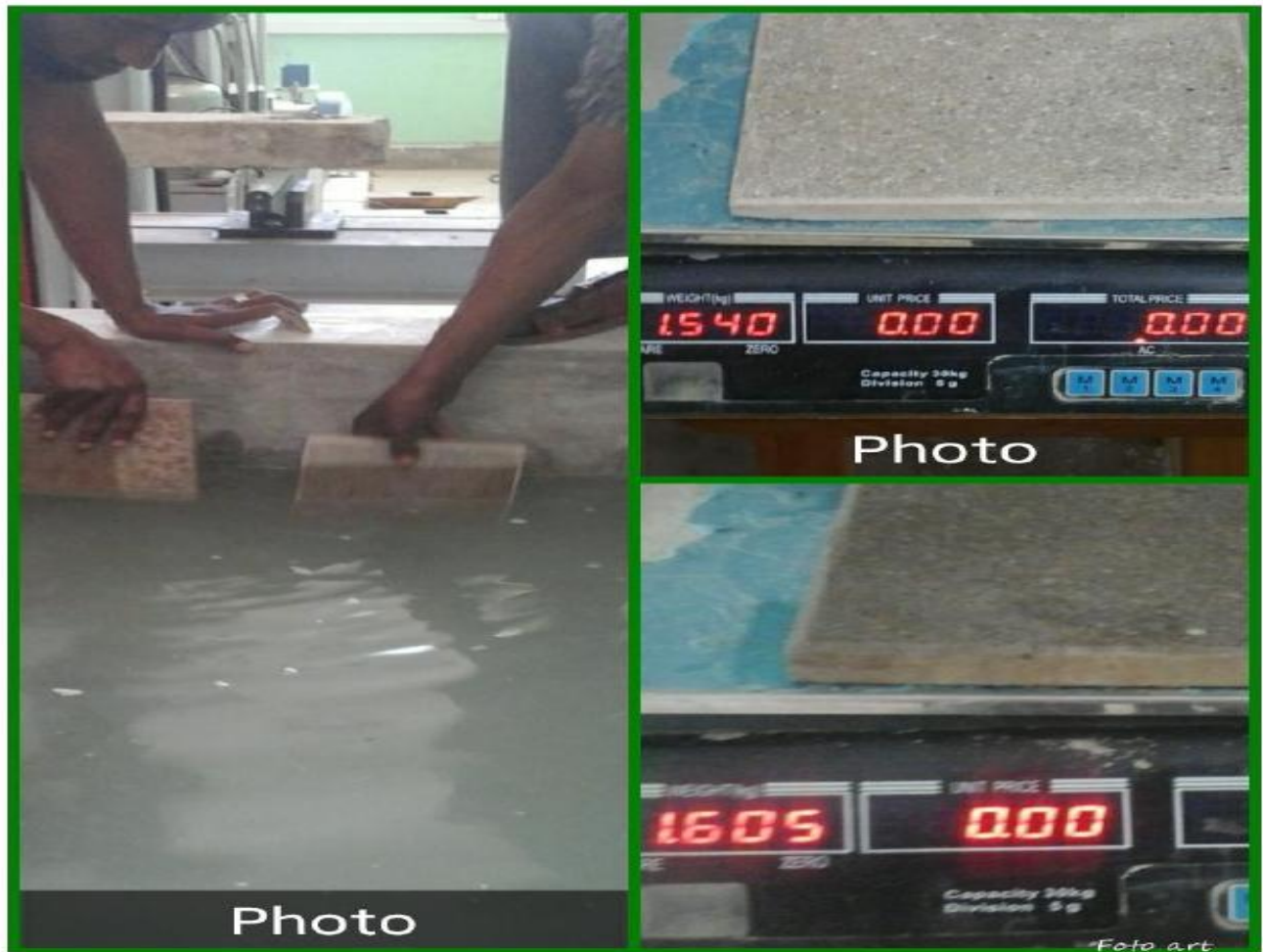
Figure 4.16 water absorption tests process
