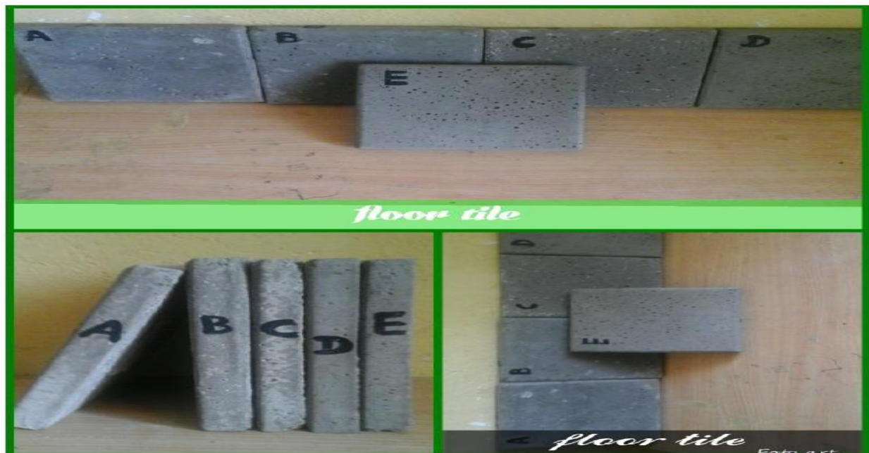
Figure 4.15 sample identification of floor tile made by waste glass aggregate as different %
