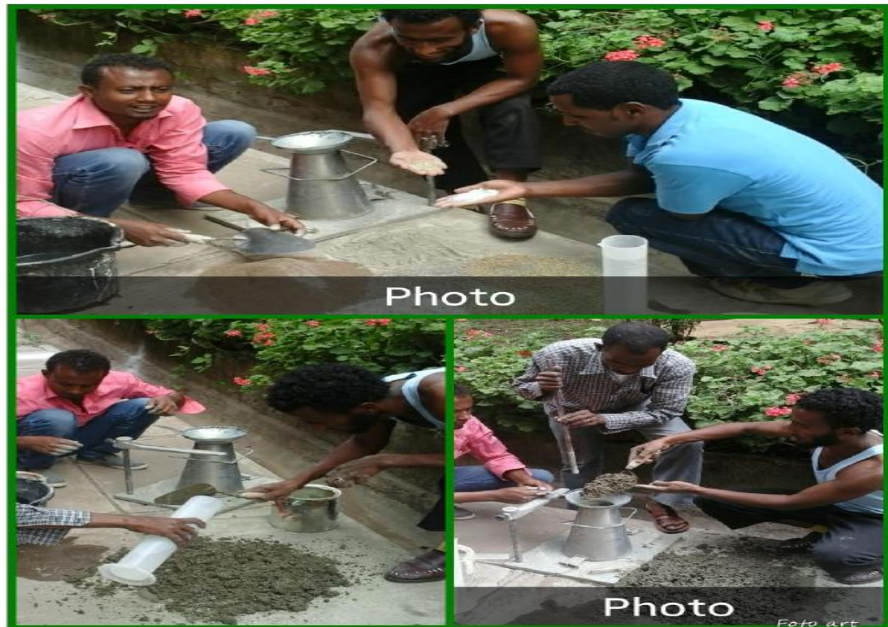
Figure 4.14 slump test process of the project
