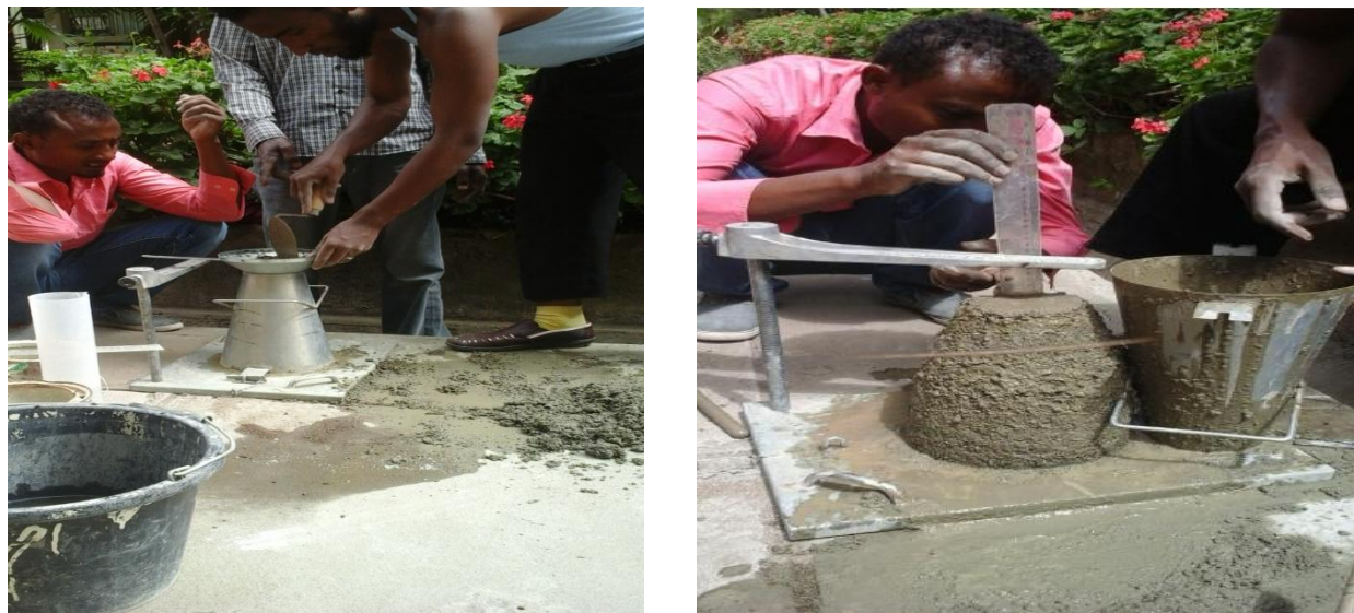
Figure 5.1 measuring of slump test
