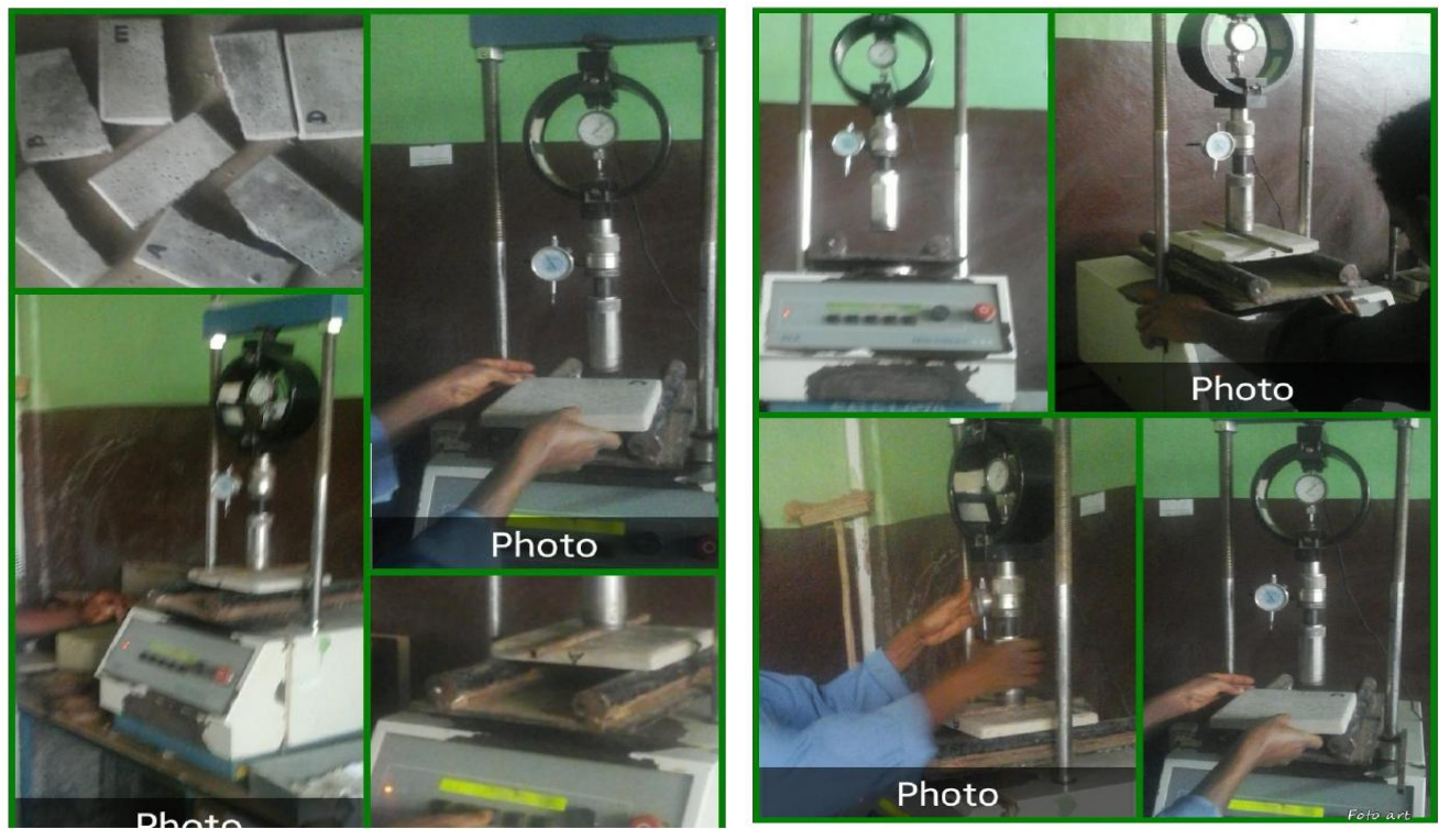
Figure 4.17 operation of compressive strength in SABA engineering laboratory.
