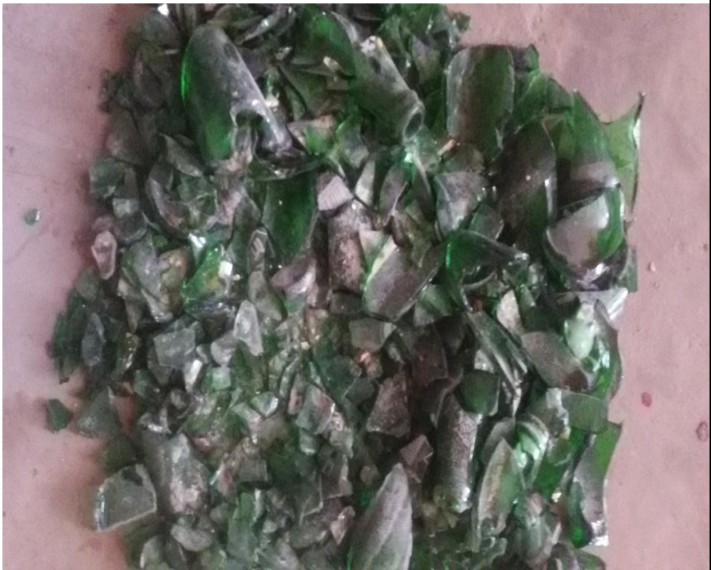
Figure 4.6 prepared green color broken bottles
