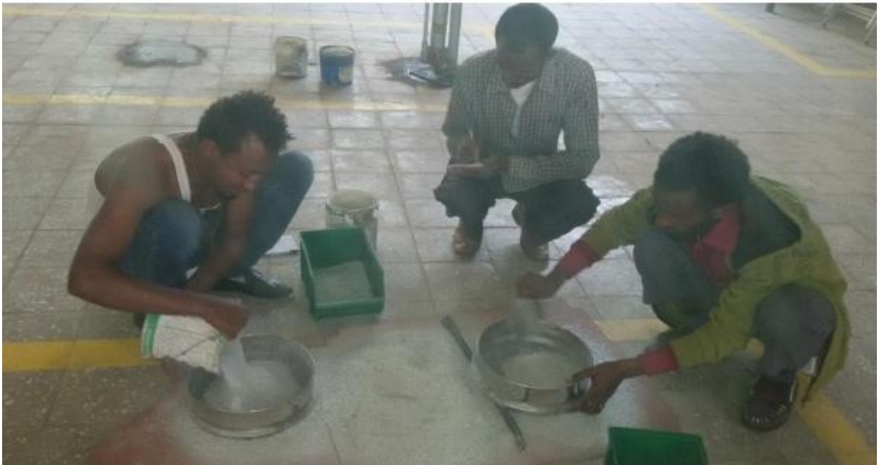
Figure 4.11 sieve analysis process
