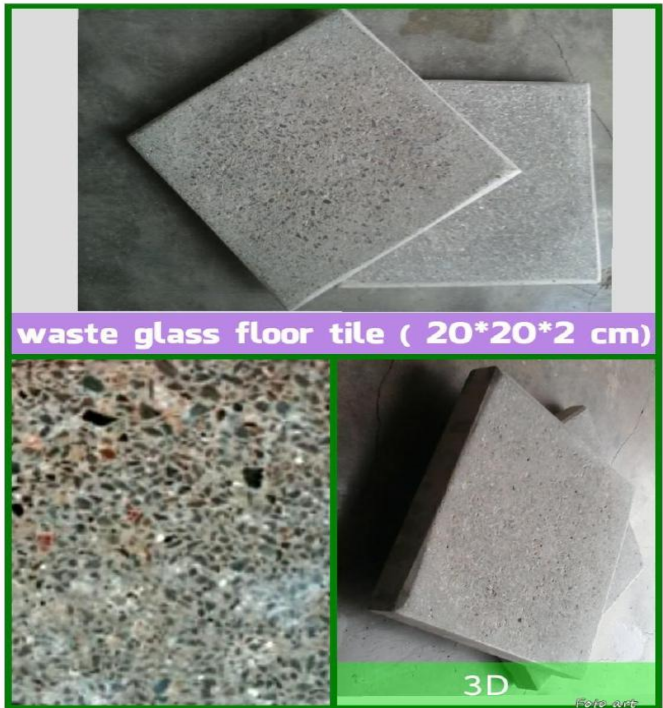
Figure 5.5 Output of the project waste glass floor tile (after grinding and finishing)
