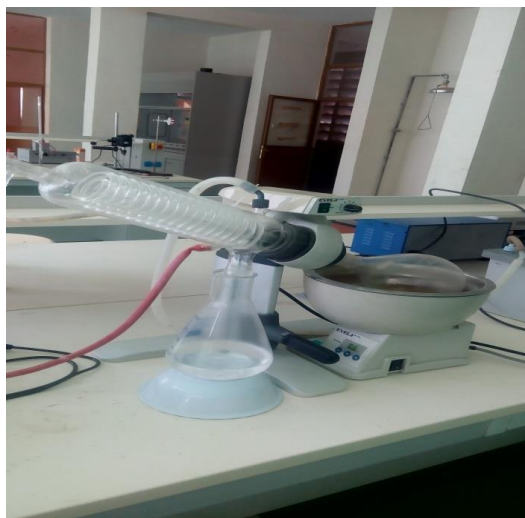
Figure 6: Rota vapour Hexane recovery
