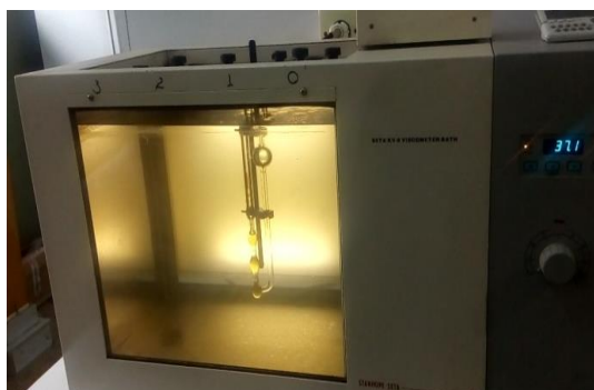
Figure19: Cannon glass Fenske capillary Viscometer Tube in a SETA.KV-8 viscometer bath
