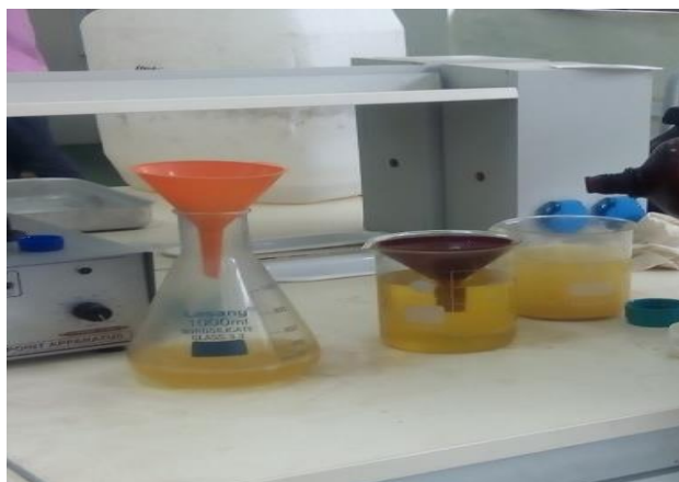
Figure 5: Filtered solution of Crude neem oil and hexane
