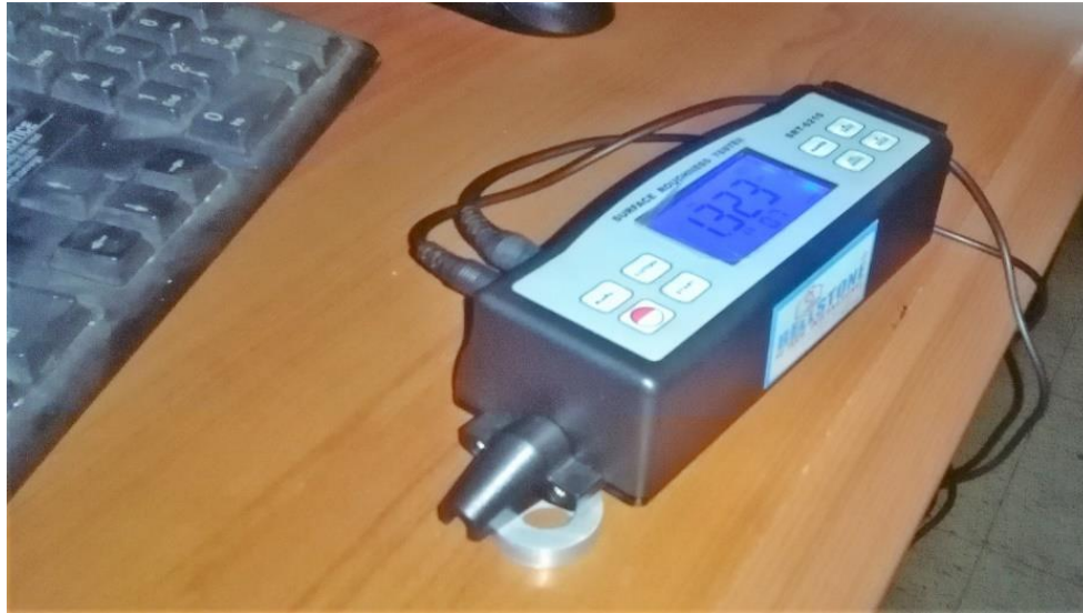
Figure 3. 4 Surface roughness tester and ring specimen setup
