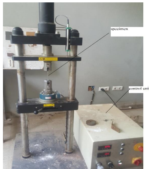
Figure 3.8 Experimental set up for plastic strain ratio test
