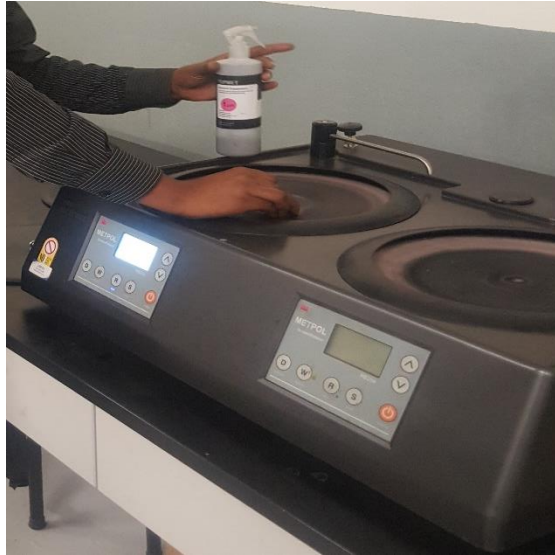
Figure 3.3 Rotating silicon carbide paper with diamond suspension
