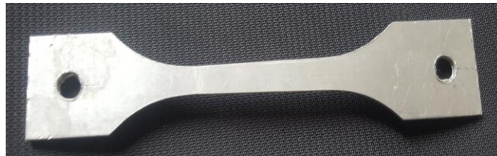
Figure 3.7 ASTM-E517 standard specimens for plastic strain ratio test
