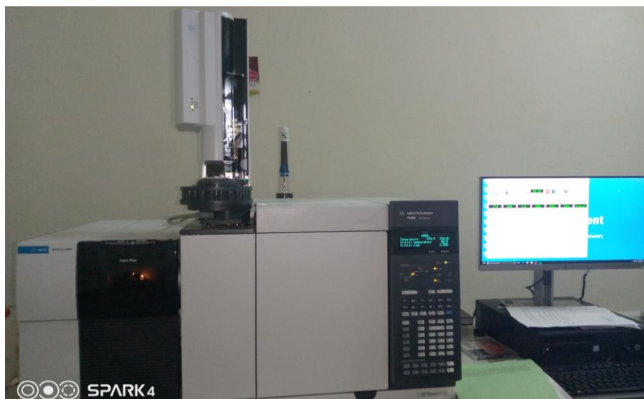
Figure 3-9: Agilent Technologies 7890B GC System used for identifying Phytochemical components.
