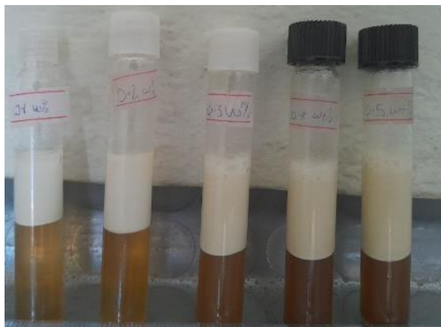
Figure 4.19 Emulsification profile of saponin with different concentration
