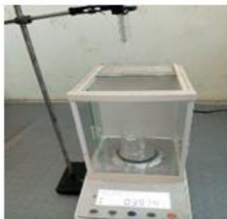
Figure 3.4 Drop-weight methods for surface tension test of saponin from P. dodecandra berry.
