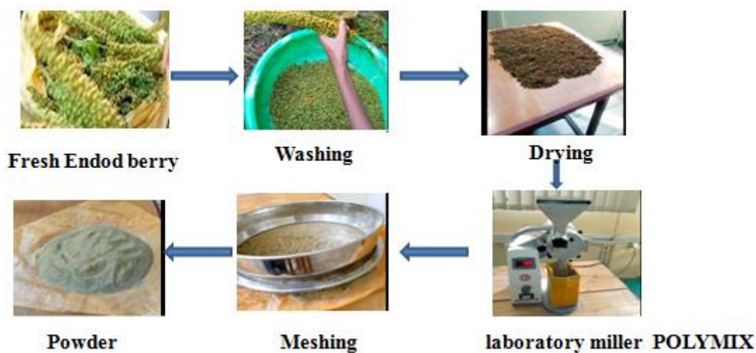
Figure 3.1 Diagrammatic representation of Endod berry powder preparation
