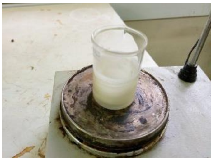
Figure 3.3 Foam formations using magnetic stirrer for 1min.
