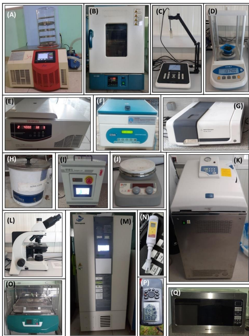
Figure: Image shows LYO60B-1S Benchtop Freeze Dryer, Bioevopeak, China (A); GX-65B Drying Oven, Huanghua Faithful Instrument Co., LTD., China (B); 1100L VWR Phenomenal pH meter (C); LA 124, VWR Electronic Beam Balance, Italy (D); TLG-16M, Drawell refrigerated Centrifuge, China (E); TC4815D MICROSPIN Centrifuge, Eltek, Maalab, India (F); Cary 60 UV-Vis, Agilent Technologies, California, U.S (G); RK106S Sonorex Ultrasonic Bath, Bandelin, Germany (H); KZ-III High Speed Tissue Homogenizer, Servicebio, China (I); MS-H280-PRO Magnetic Hotplate stirrer, DLAB, UK (J); Presoclave III Autoclave, J.P.Selecta, Spain (K); Visiscope TL524PH, VWR Microscope, Italy (L); ULF86 Ultra Low Temperature Freezer, Bioevopeak, China (M); pH Pen Tester, Bioevopeak, China (N); FS-50B Shaking Incubator, Huanghua Faithful Instrument Co., LTD., China (O); 72H, Garmin GPS, U.S (P); R-562CT(ST) Microwave, Sharp, Japan (Q).
