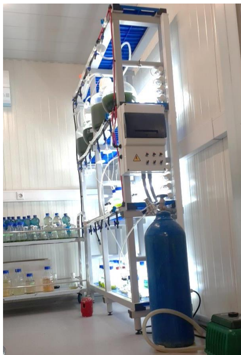
Figure 7. Laboratory setup at National Microalgae Biotechnology Laboratory, BETin for growing algal cultures.
