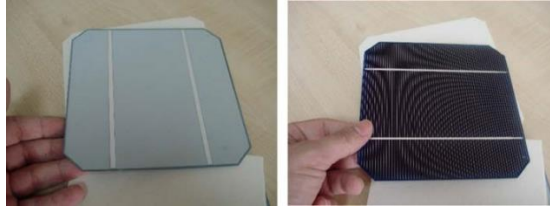
FIGURE 2. 8. A monocrystalline silicon cell's front and back (Puthenpurakel & Subadhra, 2016)
