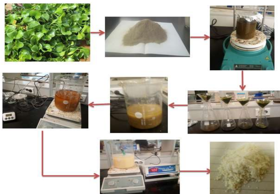
Figure 3.1: Schematics for Extraction of Cellulose from Water hyacinth
