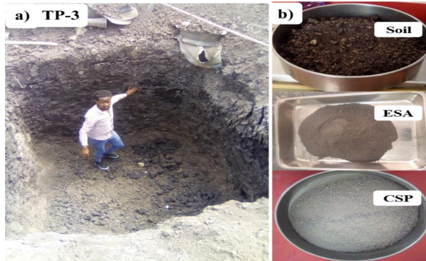
Figure 3-6: Images of (a) test pit and (b) materials used in the study
