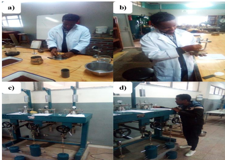
Figure 3-13: Photographic view of (a) specimen preparation (b) specimen mounted in consolidation cell (c) consolidation apparatus (d) data recording
