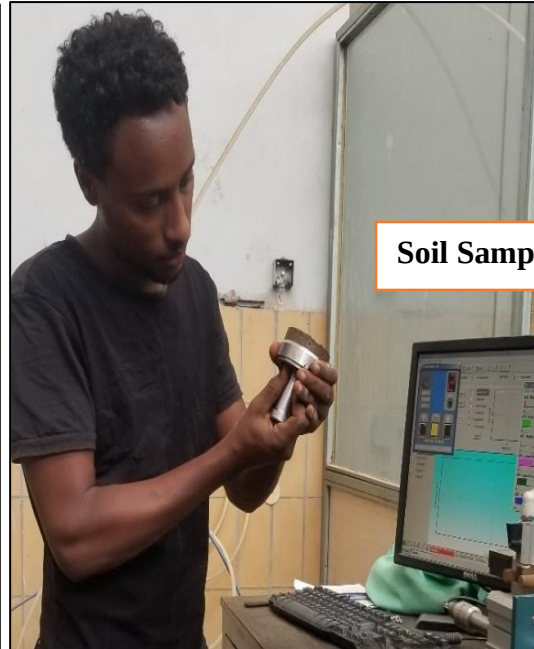
Cyclic simple shear test operation
