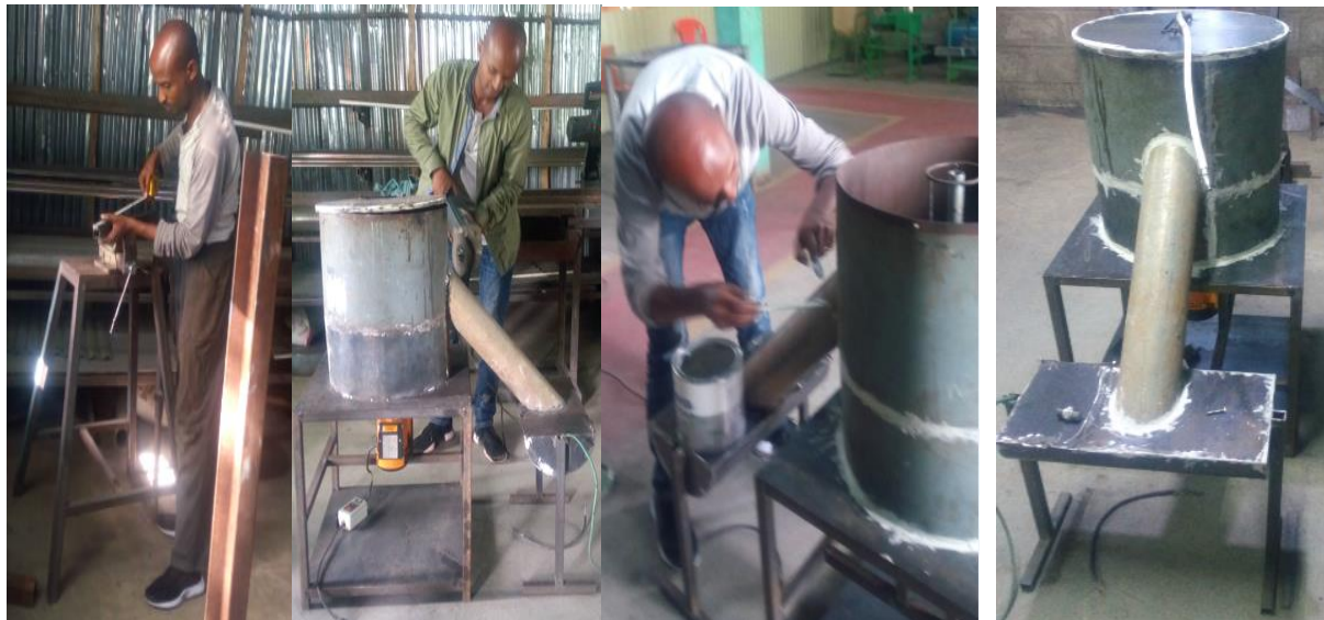
Figure 5.1 Fabrication of prototype of air filter cleaner bench.
